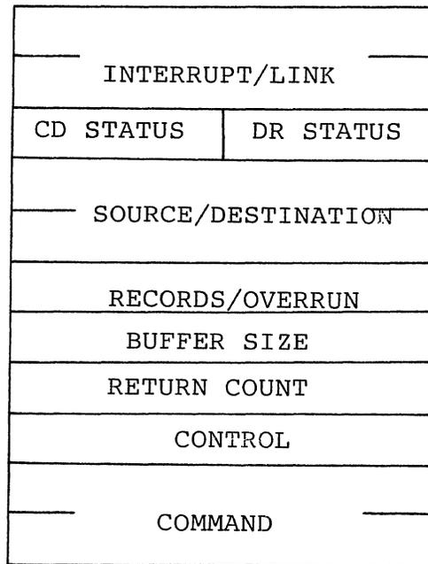
Figure 4-1 Tape Parameter Block
