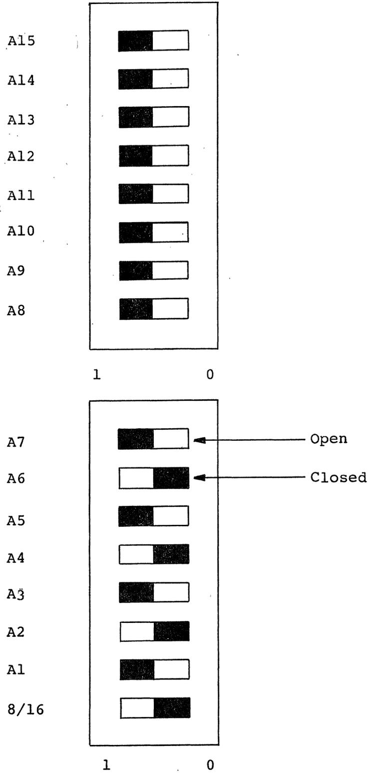
Figure D-2 Channel Attention Address 0FFAAH
