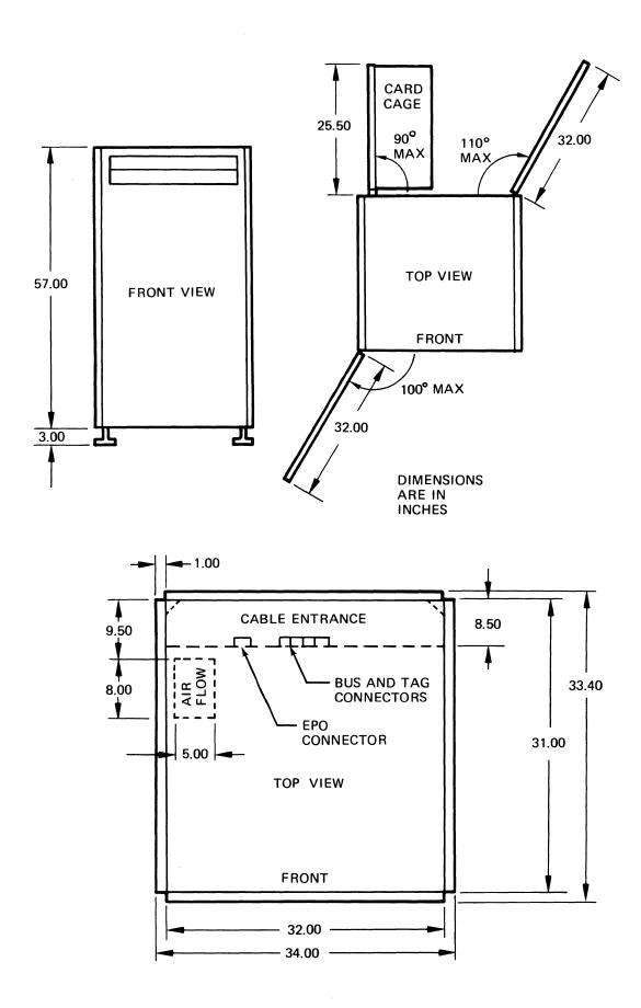
Model 1030 Controller, Installation Clearances
