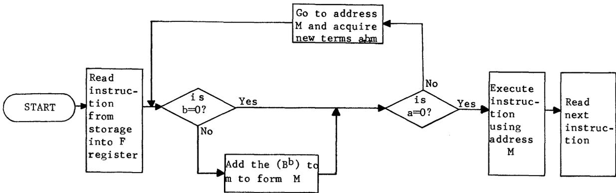
Figure 4-11. Formation of execution address (M)
