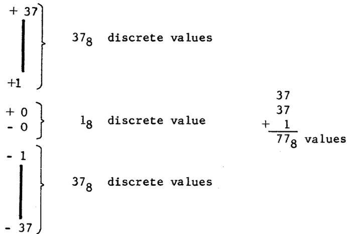
A 6-bit unsigned device could express  $100_8$  discrete values whereas a 6-bit signed device should express 1 less or  $77_8$  discrete values. Therefore, the modulus of a 6-bit unsigned device would be expressed as  $2^6$  but the modulus of a 6-bit signed device would be expressed as  $2^6 - 1$  ( $2^6 = 100_8$ ,  $2^6 - 1 = 77_8$ ). A 24-bit signed device would have a modulus of  $2^{24} - 1$  and a 24-bit unsigned device would have a modulus of  $2^{24}$ .
