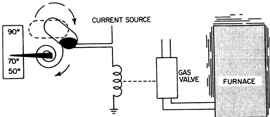
Now you manually readjust thermostat to 50° - switch opens - valve closes - furnace goes off.
