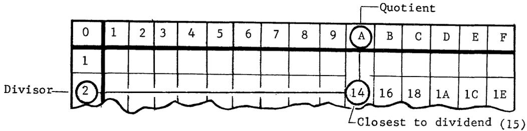
$$\begin{array}{r} A \\ 2 \overline{) 15} \\ \underline{14} \\ 1 \end{array}$$
