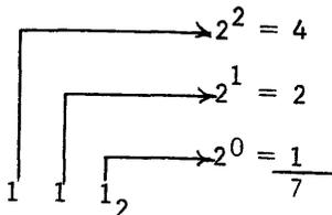
A 1 in the  $2^2$  position would have a decimal equivalent of  $2^2$  or 4, whereas a 1 in the  $2^1$  position would have half that value ( $2^1$  or 2).
