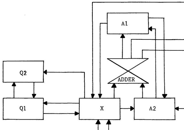
Figure 4-15. Arithmetic Section
