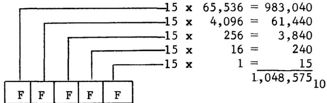
Remember, the radix of the device was 16, so the value of each positional character is 16 times the value of the character immediately to its right.
