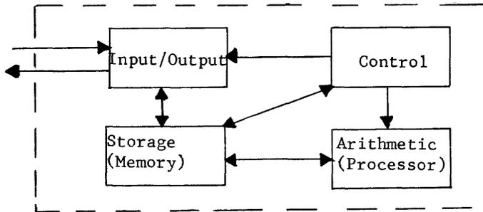
By the previous definitions, it should be apparent that all four sections are necessary to an automatic computer. The dotted lines around the four sections are the outer dimensions of an automatic computer.
