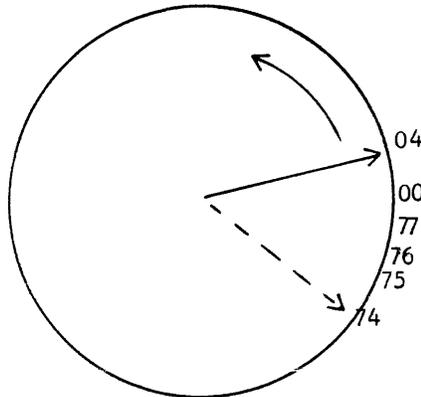
The pointer now indicates an answer of  $74_8$ . Any time the upper octal digit is four or greater, the signed binary equivalent would indicate a negative operand. Recomplement to find the true value and attach the negative sign.
