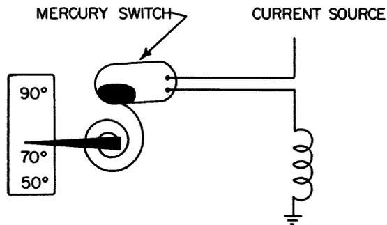
Temperature drops to 72° - coiled spring retracts - opens gas valve - furnace comes on - temperature rises.
