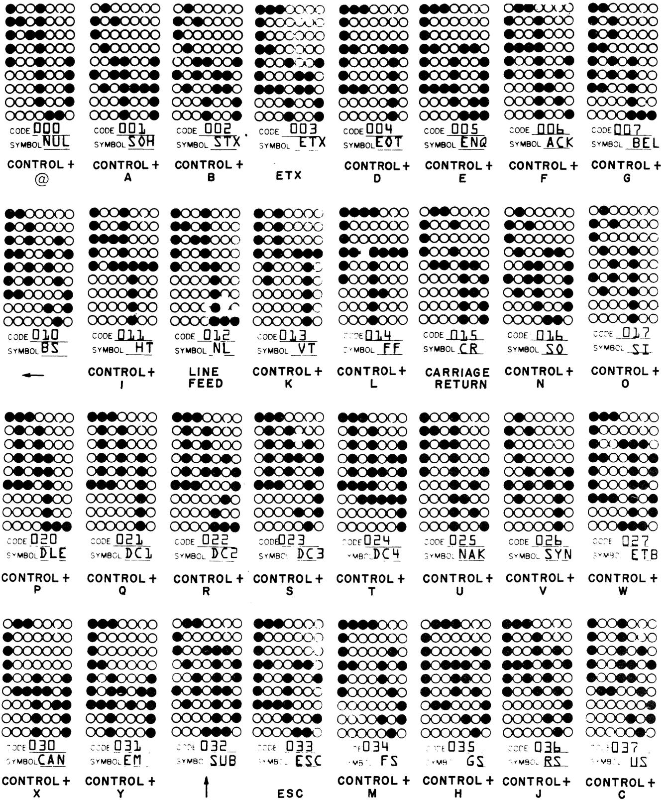
Figure 4-2. Control Code Dot-Matrix Formations and Octal Codes\*
