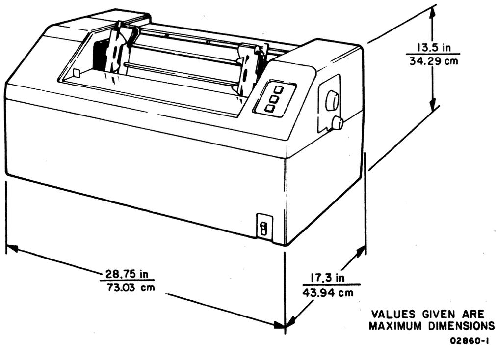
Figure C1-2. 70-LPM Impact Printer Dimensions
