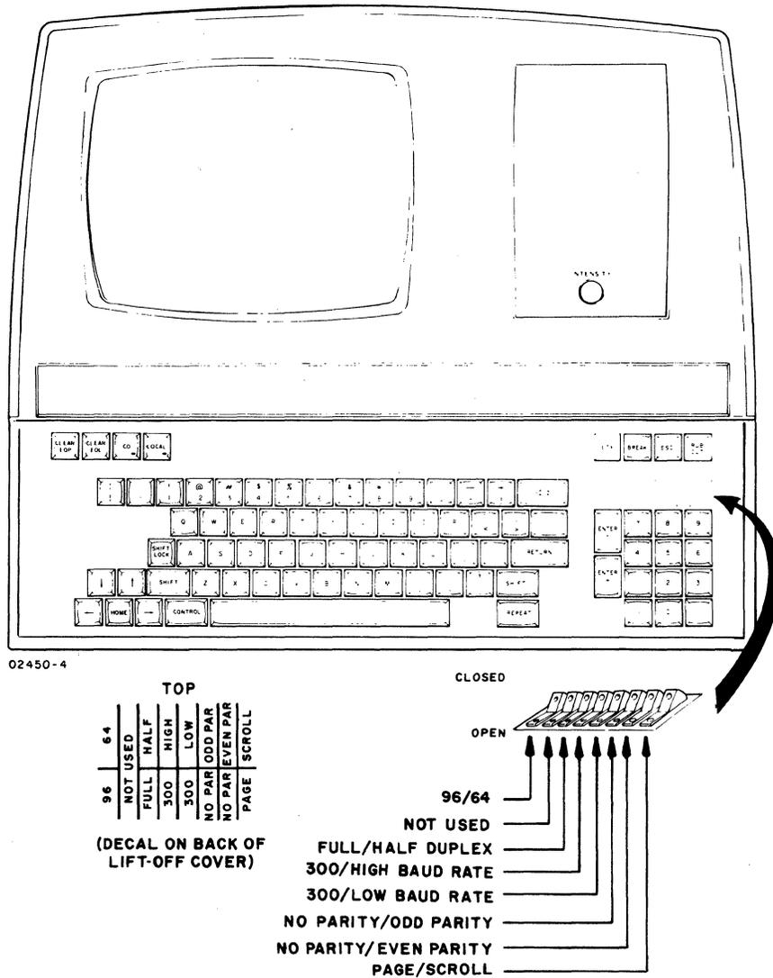
Figure D-2. 82-Key Keyboard and Operator-Control Features
