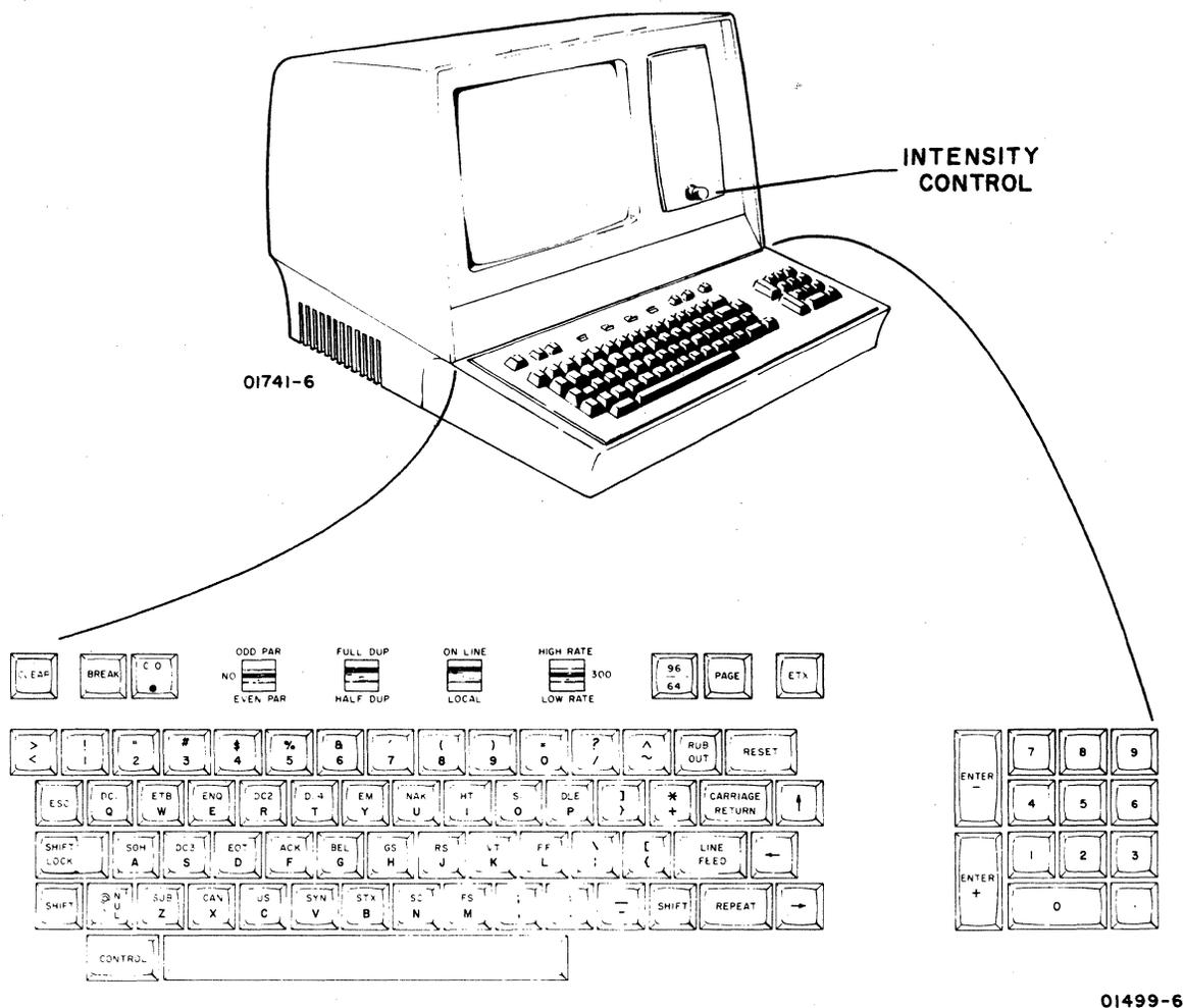
Figure 2-3. External Controls, Keyboard and Front Panel
