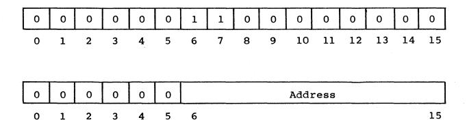
This command causes the rigid-disk adapter to jump to location  $A_6 \cdot \cdot \cdot A_{15}$  of the interface RAM. The code to be executed must be NEED CORRECT TERM MP100-type object code. This command is useful for writing patches and executing some diagnostic routines.
