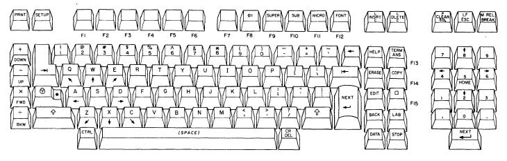
Figure B-1. Type 3 Terminal Keyboard with Standard English Keycaps
