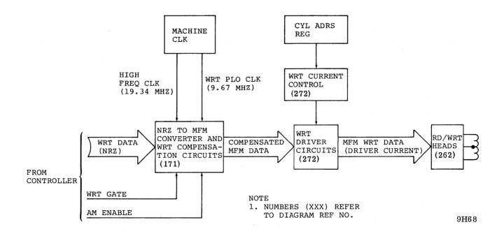
Figure 3-47. Write Circuits - Block Diagram
