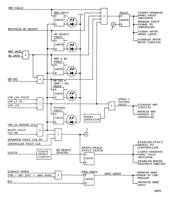
Figure 3-59. Fault and Error Detection
