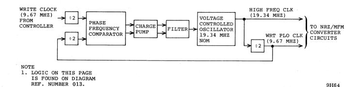
Figure 3-39. Write Clock Multiplier
