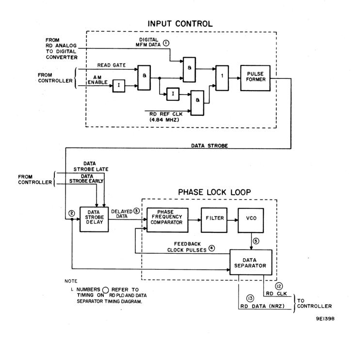
Figure 3-56. Read PLO and Data Separator Circuits
