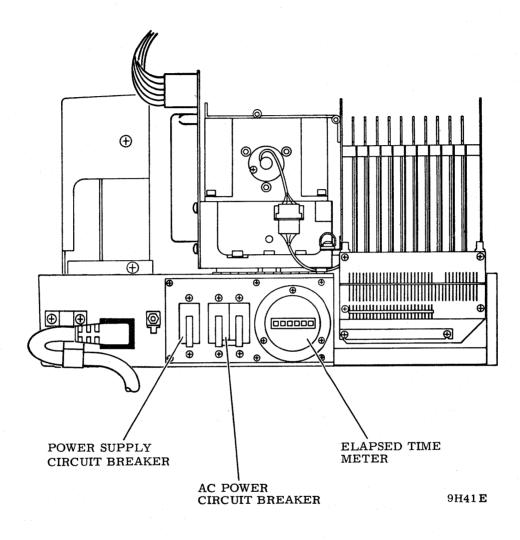
Figure 2-2. Power Control Panel Switches and Indicators
