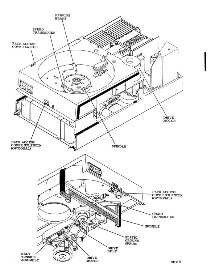
Figure 3-7. Disk Pack Rotation Mechanisms
