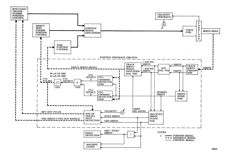
Figure 3-21. Position Feedback Circuit - Block Diagram
