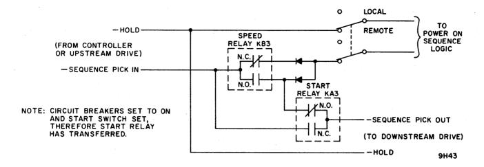
Figure 3-3. Power Sequencing Circuits
