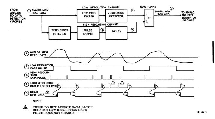
Figure 3-54. Read Analog to Digital Converter - Logic and Timing
