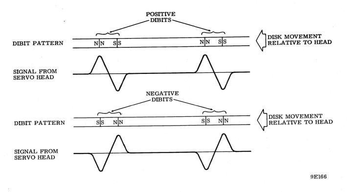
Figure 3-18. Positive and Negative Dibit Pattern
