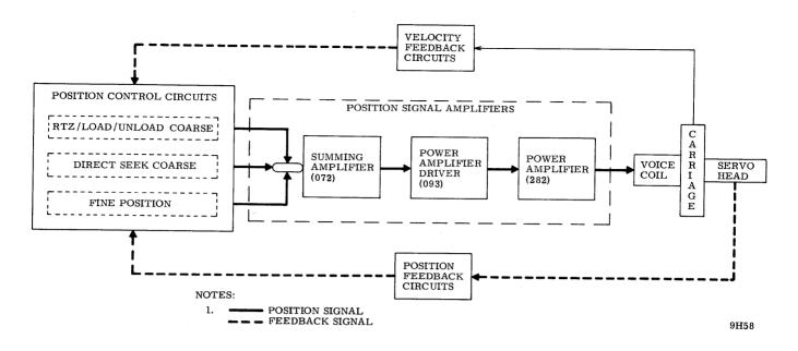
Figure 3-28. Position Signal Amplifier Circuits
