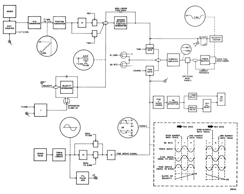
Figure 3-16. Servo System Functional Block Diagram
