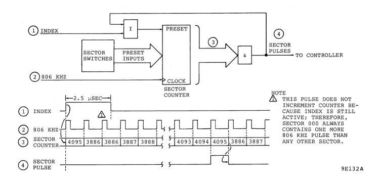
Figure 3-45. Sector Detection - Logic and Timing
