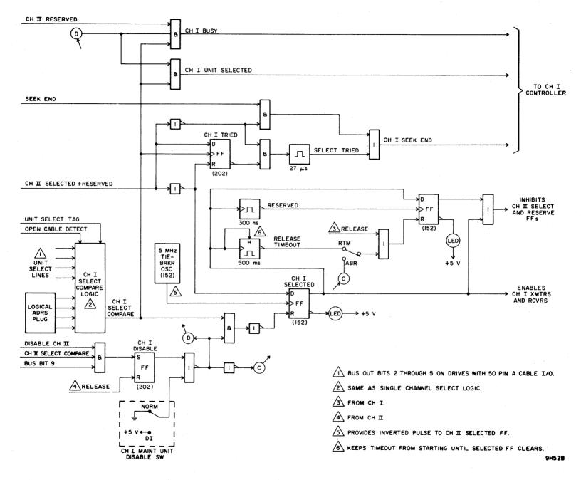
Figure 3-14. Channel I Dual Channel Select Logic
