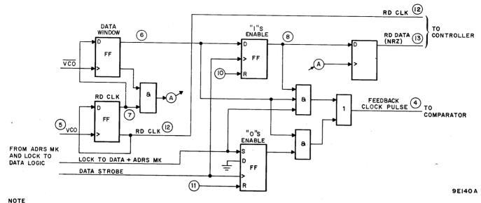
I. NUMBERS O REFER TO TIMING ON RD PLO AND DATA SEPARATOR TIMING DIAGRAM.
