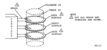
Figure 3-20. Cylinder Concept
