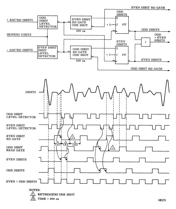
Figure 3-24. Odd/Even Dibit Clock - Logic and Timing
