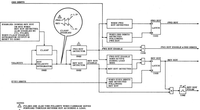
DETECTORS ENABLED WHENEVER DISK IS UP TO SPEED EXCEPT DURING HEADS UNLOAD.
