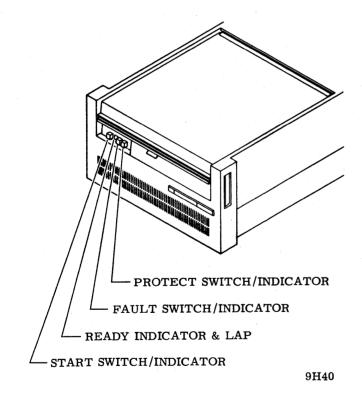
Figure 2-1. Control Panel Switches and Indicators
