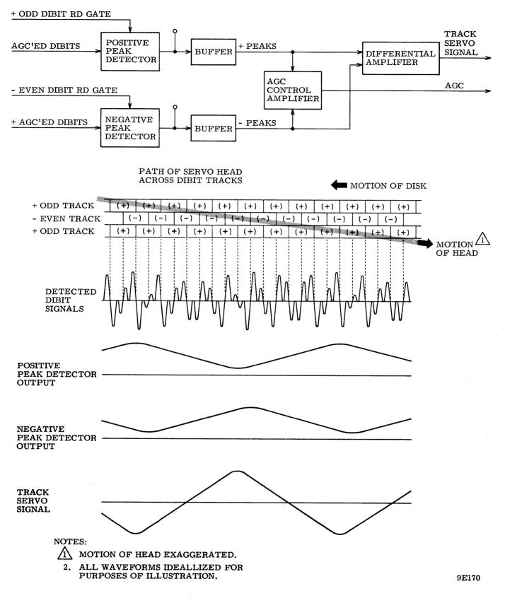
Figure 3-23. Track Servo Amplifier Circuit and Signals
