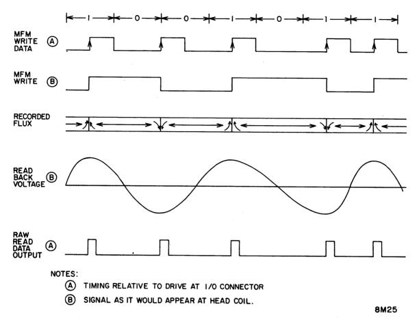
Figure 3-48. MFM Recording - Waveforms and Timing
