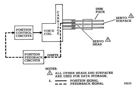
Figure 3-17. Servo Head and Surface
