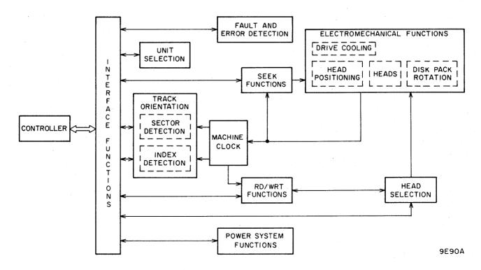
Figure 3-1. Drive Functional Block Diagram
