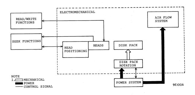
Figure 3-6. Electromechanical Functions - Diagram Block
