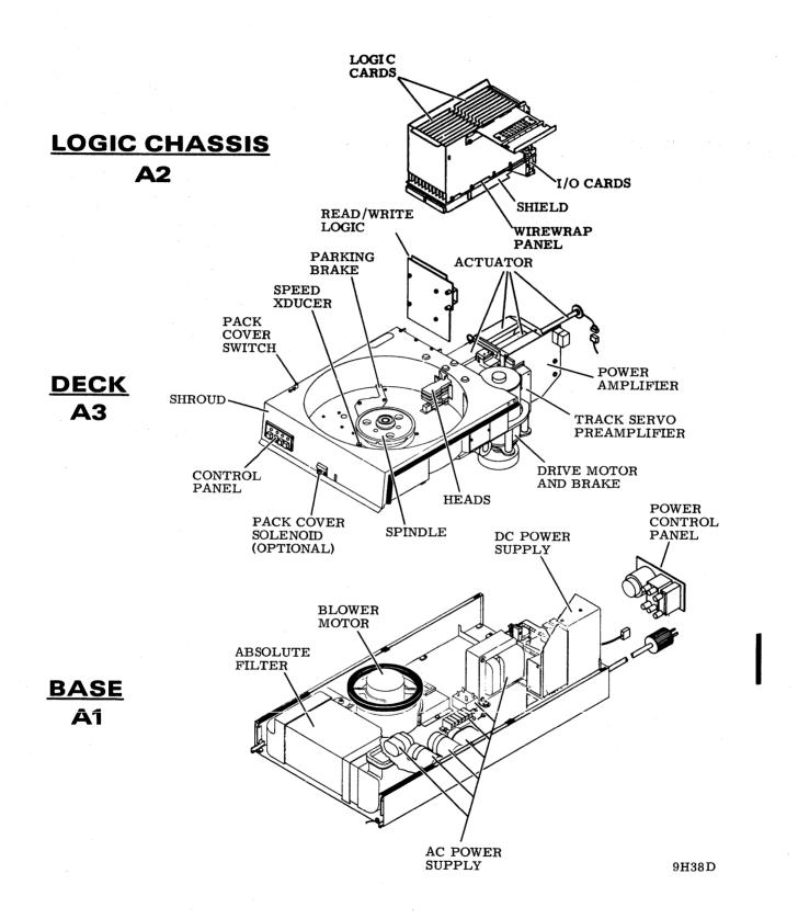
Figure 1-4. Drive Electronics Package
