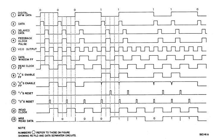
Figure 3-58. Read PLO and Data Separator Timing
