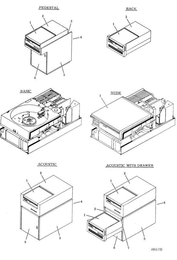
Figure 1-3. Drive Mounting Configurations
