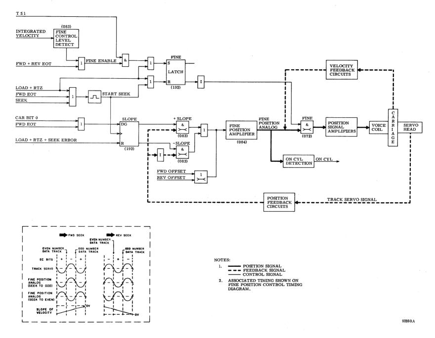
Figure 3-31. Fine Position Control Circuits
