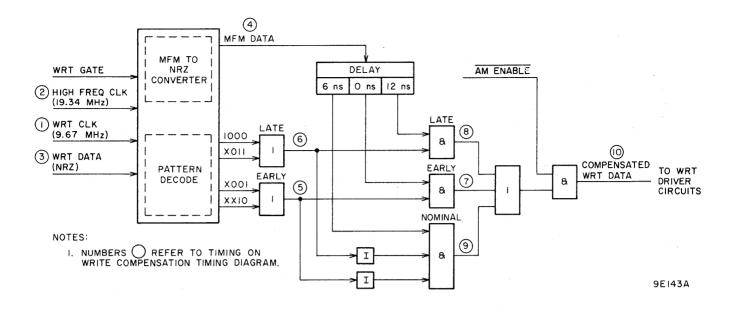
Figure 3-49. NRZ to MFM Converter/Write Compensation Circuit
