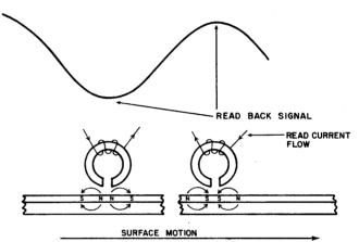
NOTE: RELATIVE HEAD TO SURFACE MOTION, REPRODUCING (READ OPERATION) 7518A
