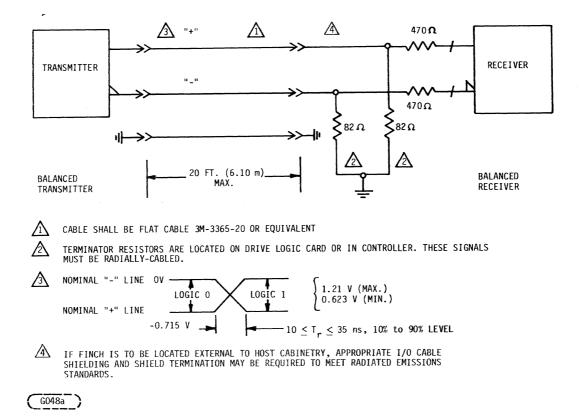
Figure 14. Balanced Differential Drivers/Receivers
