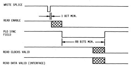
READ ENABLE MUST BE DEACTIVATED PRIOR TO THE WRITE SPLICE. READ ENABLE MAY BE REINITIATED AT LEAST ONE BIT AFTER THE WRITE SPLICE AND WITH AT LEAST 11 BYTES OF PLO SYNC REMAINING IN THE SYNC FIELD.
