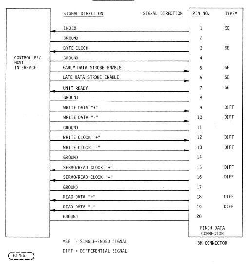
Figure 16. Data Cable Interface
