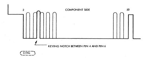
Figure 12. Command Cable Interface
