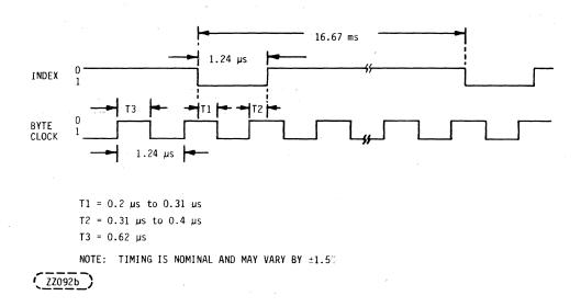
Figure 21. Index and Byte Clock Relationship
