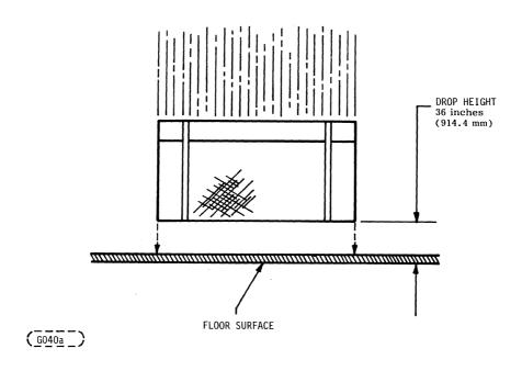
Figure 6. Flat Drop Test
