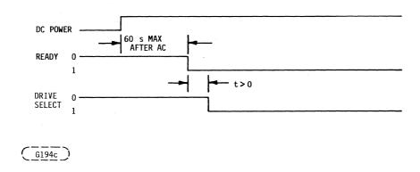
Figure 17. Power Turn On and Drive Selection
