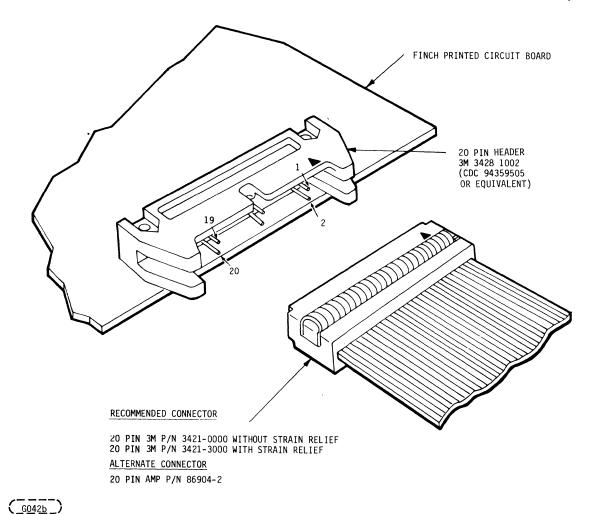
Figure 11. Data Cable Interface
