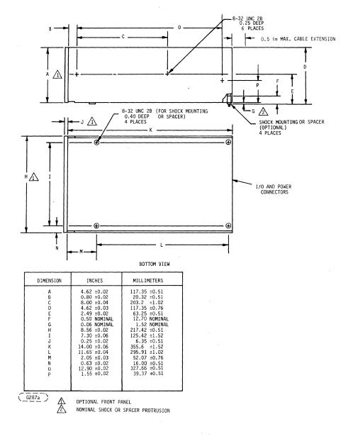
Figure 7. Mounting Configuration Dimensions
