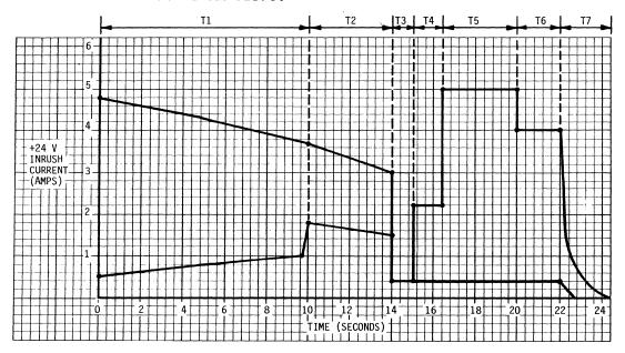
Figure 4. Typical +24VDC Current Profile
