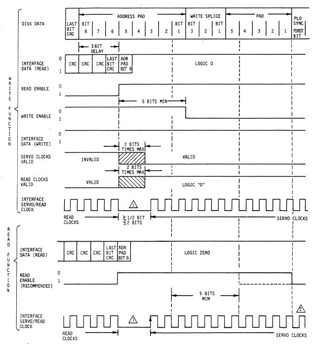
WHEN READ ENABLE IS DEACTIVATED, THE INTERFACE SERVO/READ CLOCK LINE WILL CONTAIN VALID SERVO CLOCKS WITHIN ONE HALF OF A SERVO CLOCK PERIOD MINIMUM TO 2 SERVO CLOCK PERIODS MAXIMUM. THIS TRANSITION AREA WILL NOT CONTAIN ANY SHORTENED PULSE WIDTHS, BUT IT MAY CONTAIN NO TRANSITIONS FOR UP TO TWO CLOCK PERIODS MAXIMUM.
