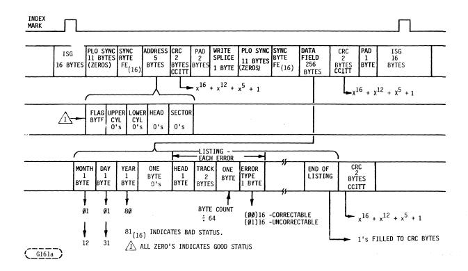
Figure 8. Format for Surface 0, Track 604, Sector 0--Factory Flagged Track Data Track
