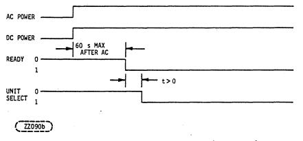
Figure 16. Power Turn On and Unit Selection
