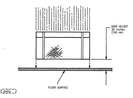
Figure 6. Flat Drop Test
