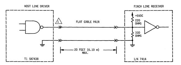
INTERFACE SIGNAL LEVELS AND LOGICAL SENSE AT THE FINCH I/O CONNECTOR ARE DEFINED AS FOLLOWS:
