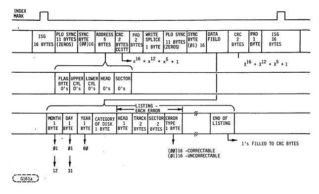
Figure 8. Format for Surface 0, Track 0, Sector 0--Factory Flagged Track Data Track
