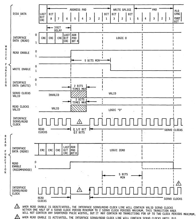
WHEN READ ENABLE IS ACTIVATED, THE INTERFACE SERVO/READ CLOCK LINE WILL CONTAIN SERVO CLOCKS UNTIL PLO SYNCHRONIZATION IS ESTABLISHED. THE TRANSITION FROM SERVO CLOCKS TO READ CLOCKS WILL BE ACCOMPLISHED IN THE SAME MANNER DESCRIBED IN NOTE A, i.e., NO TRANSITIONS FOR UP TO TWO CLOCK PERIODS MAXIMUM, ETC.
