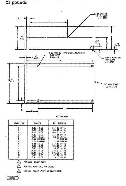
Figure 7. Mounting Configuration Dimensions
