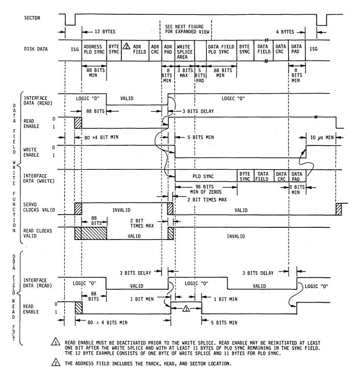
Figure 23. Typical Read/Write Timing
