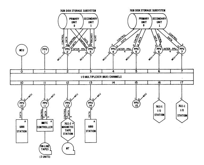
Figure II-6.2. Diagram of Typical Configuration
