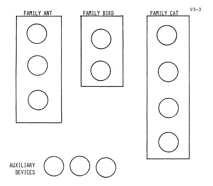
EACH 'DEVICE' WITHIN A FAMILY OR AUXILIARY DEVICE MAY BE 1 TO 8 DISK SPINDLES. EACH AUXILIARY DEVICE MAY BE DECLARED
