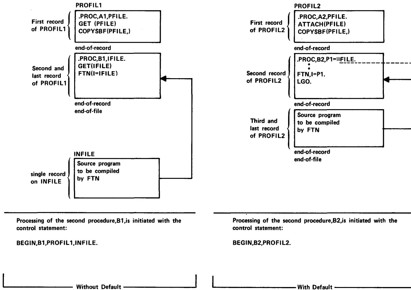
Figure 1-4-1. Procedure Access of a Data Record
