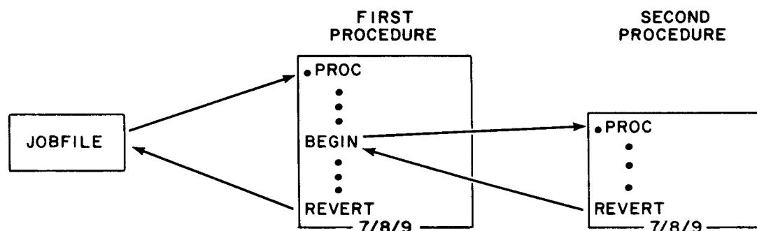
Figure 1-4-4. Calling a Procedure from Another Procedure
