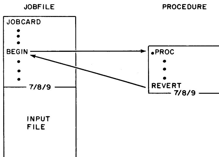
Figure 1-4-3. Calling a Procedure from a Job
