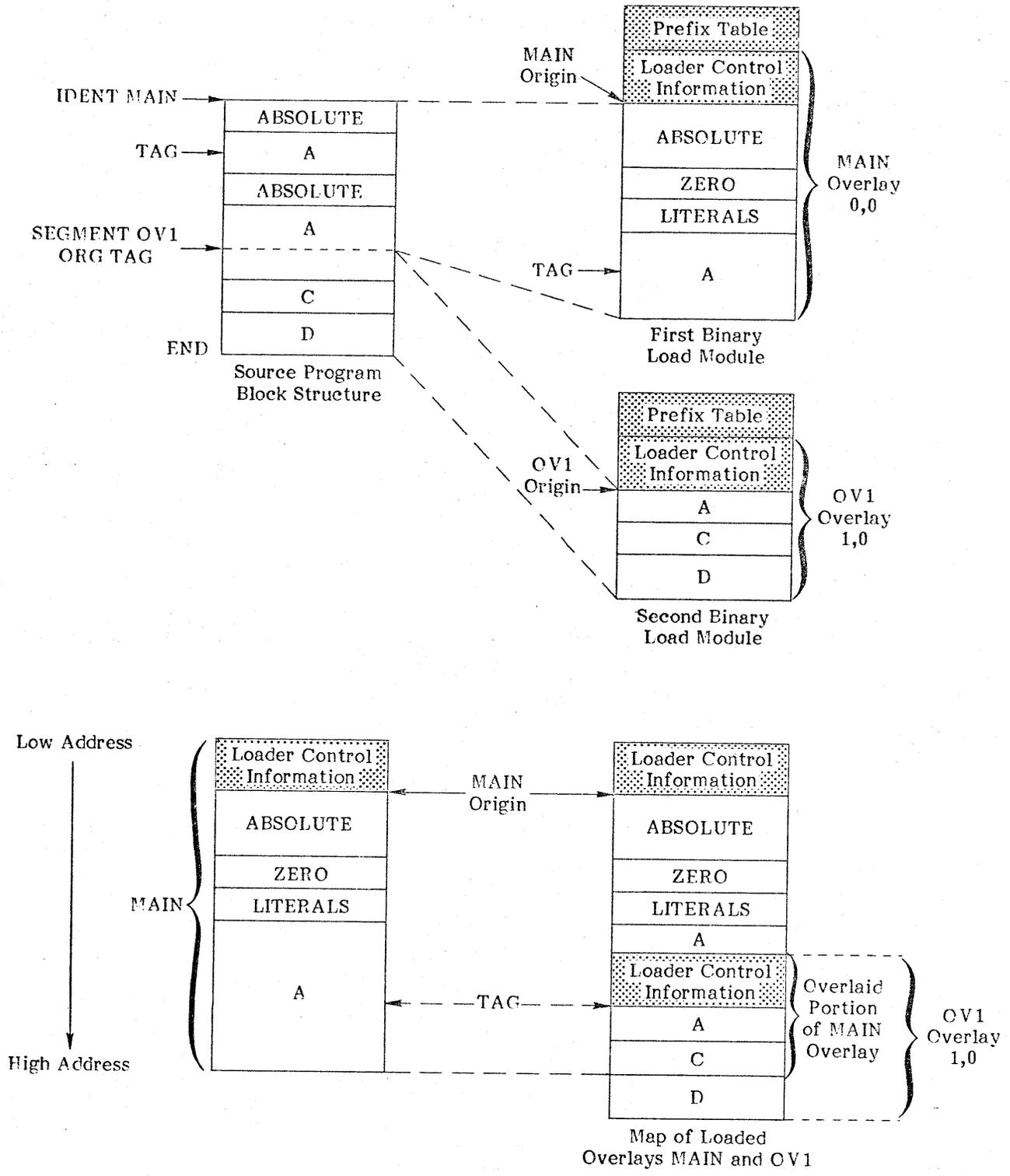
Figure 3-5. SEGMENT-Type Overlay Structure
