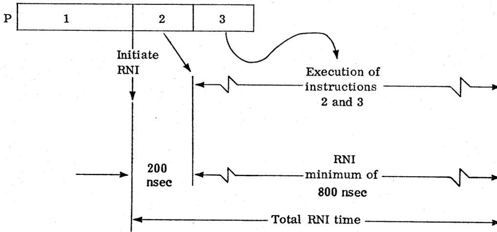
In calculating execution times, two minor cycles are added to each instruction word in a program to cover the RNI initiation time. Exceptions are the return jump and the jump instructions (in which the jump condition is met) when they occupy the upper position of the instruction word. Since the times for these instructions already include the time required to read the new instruction word at the jump address, no additional time is consumed.
