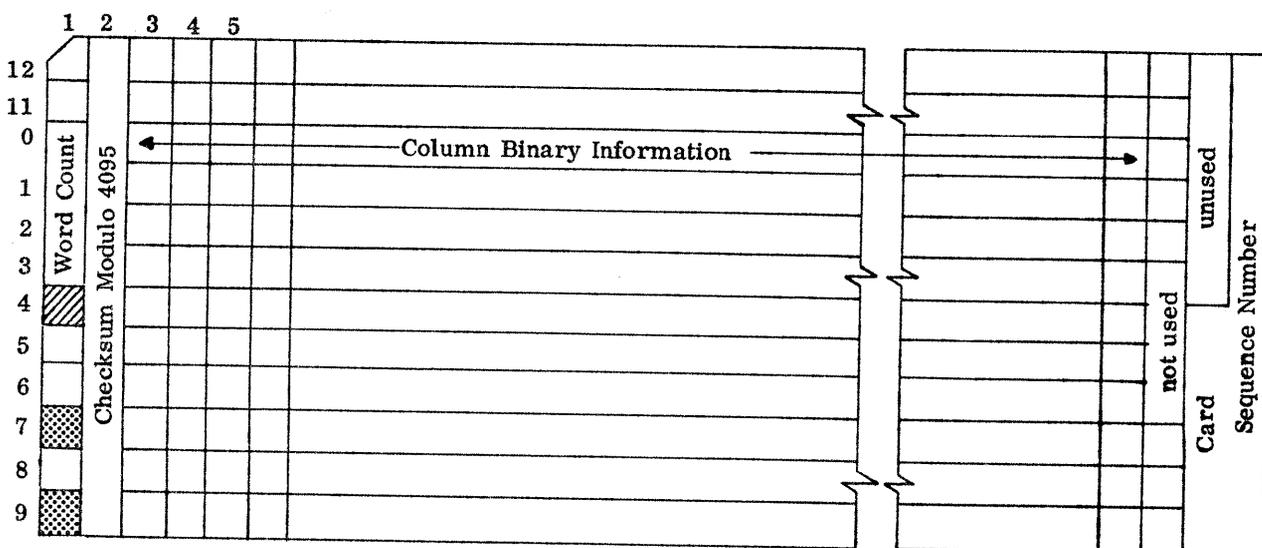
A binary card can contain up to 15 60-bit CPU words starting at column 3. Column 1 also contains a count of 60-bit words in rows 0, 1, 2, and 3 plus a check indicator in row 4. If row 4 of column 1 is zero, column 2 is used as a checksum for the card on input; if row 4 is one, no check is performed on input.
