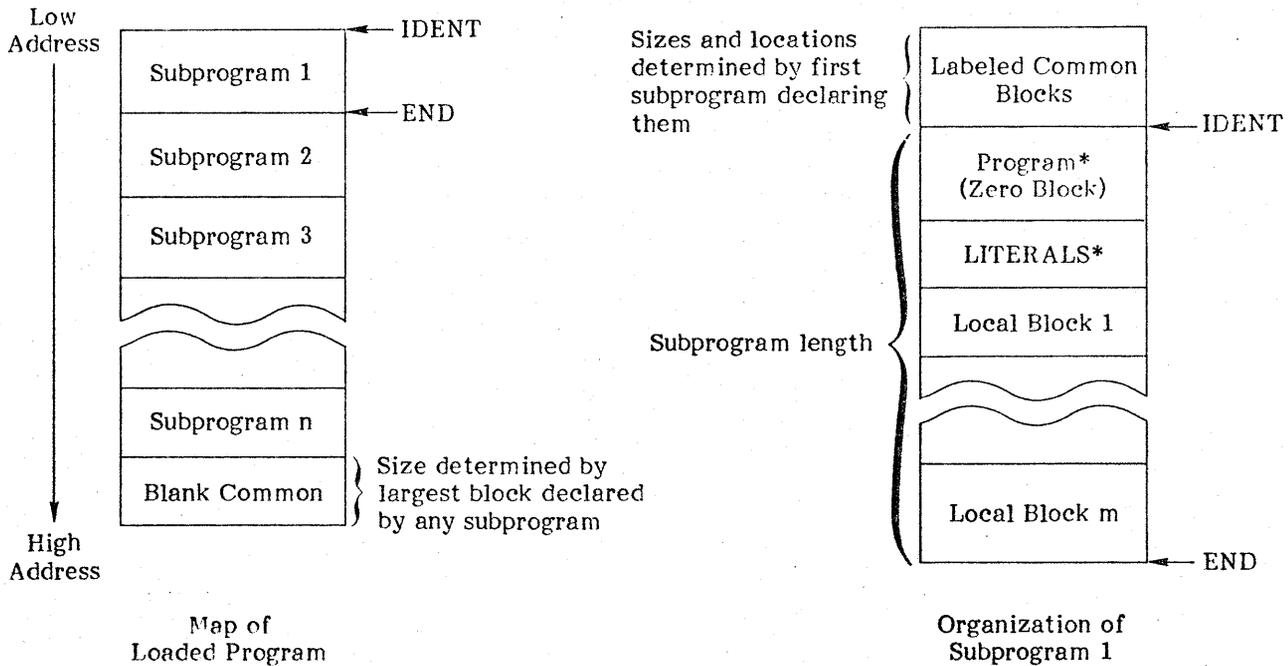
Figure 3-1. Relocatable Program Structure
