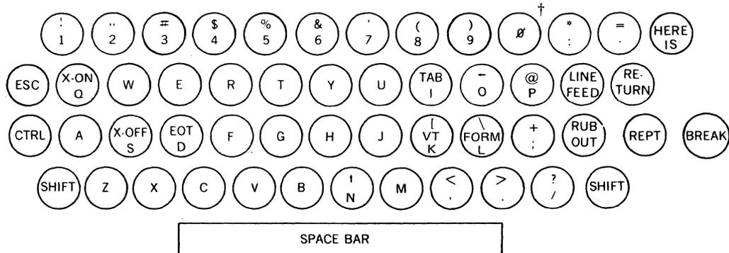
Figure F-4. Typical Model 33/35 Teletype Keyboard
