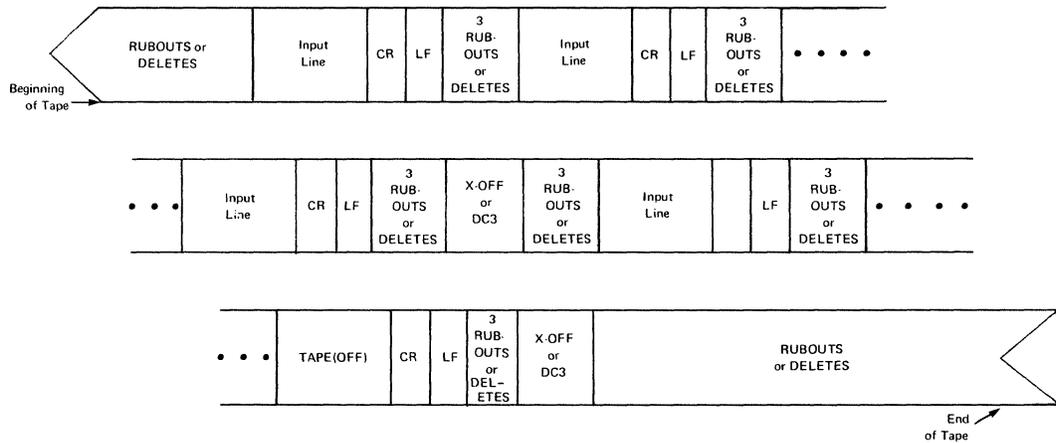
Figure F-6. Punched Tape Format
