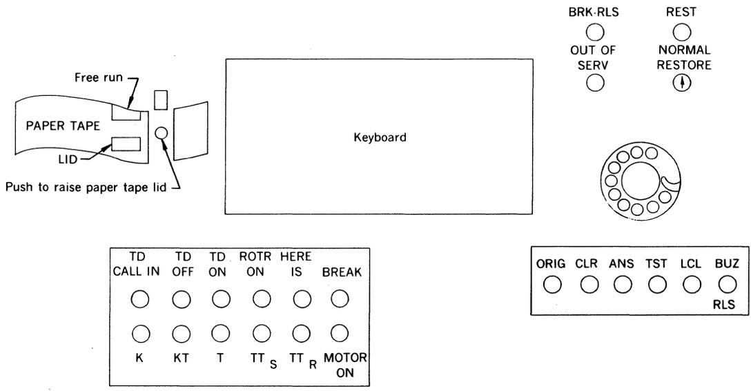
Figure F-2. Model 35 Teletype Operating Controls
