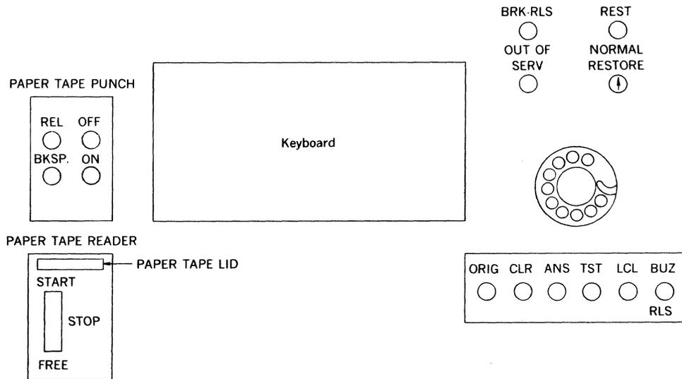
Figure F-1. Model 33 Teletype Operating Controls
