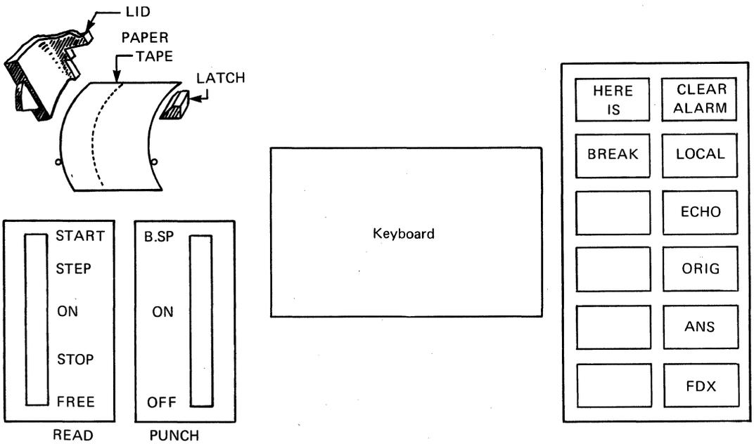
Figure F-3. Model 38 Teletype Operating Controls
