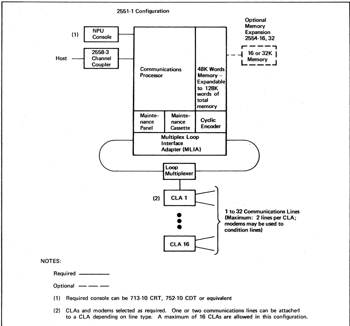
Figure 1-8. Typical NPU and Peripheral Hardware Configuration
