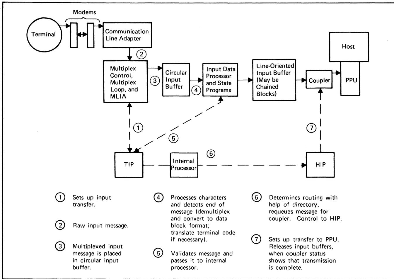
Figure 1-6. Simplified Input Message Processing
