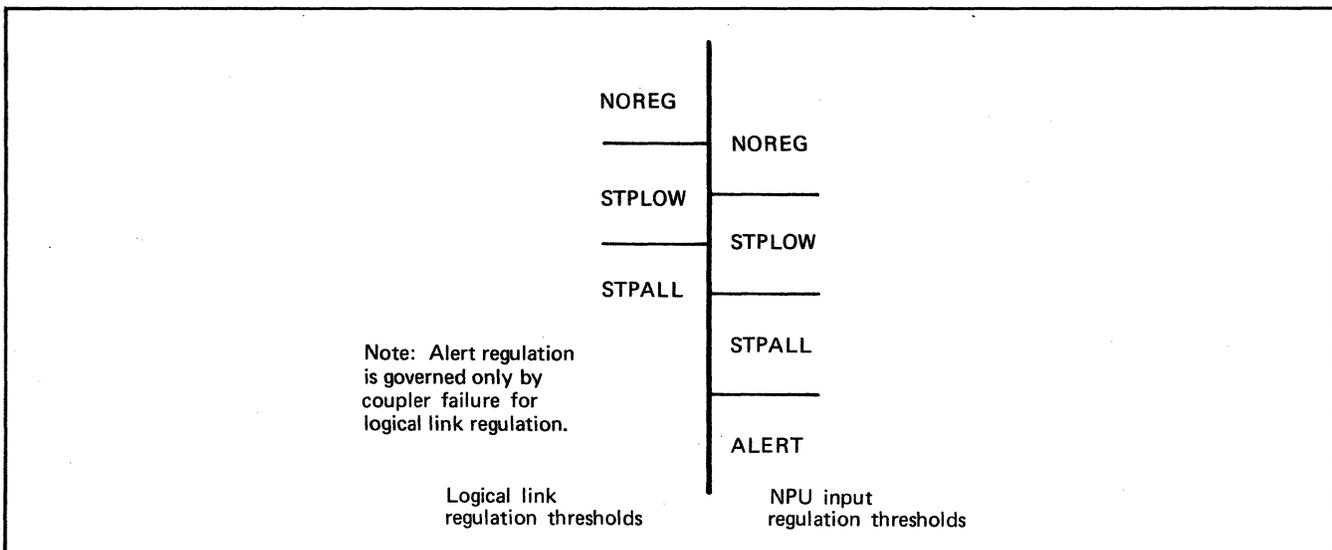
Figure 2-4. Buffer Availability Threshold Levels for Regulation
