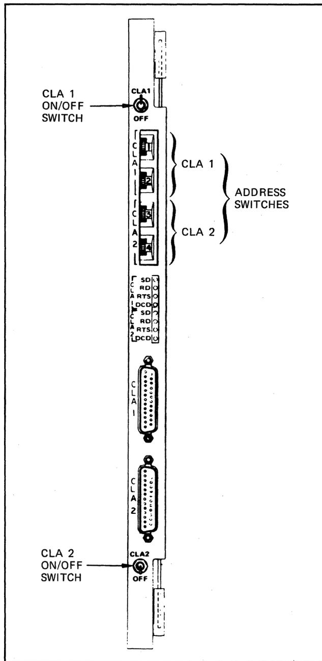
Figure 5-2. CLA Circuit Card ON/OFF Switch Location
