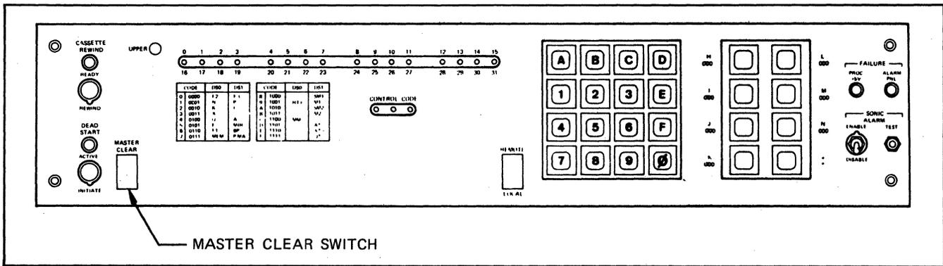
Figure 5-4. Maintenance Panel MASTER CLEAR Switch Location
