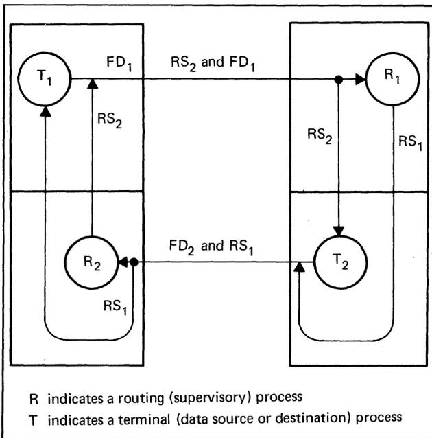
Figure H-1. Communications Paths for Block Flow Control
