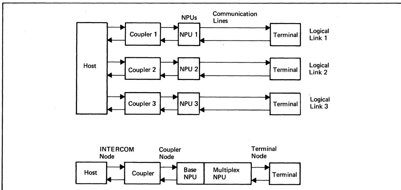
Figure 2-3. Sample Logical Link Connections
