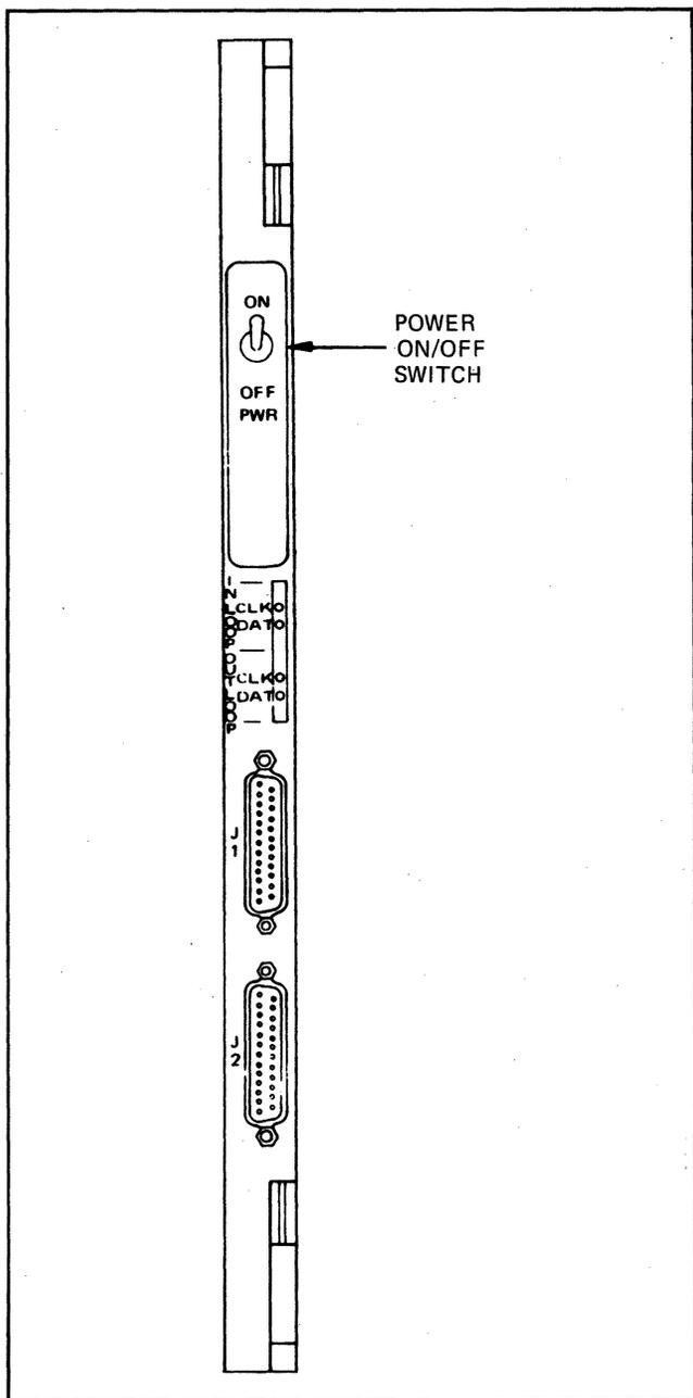
Figure 5-1. Loop Multiplex Circuit Card PWR ON/OFF Switch Location
