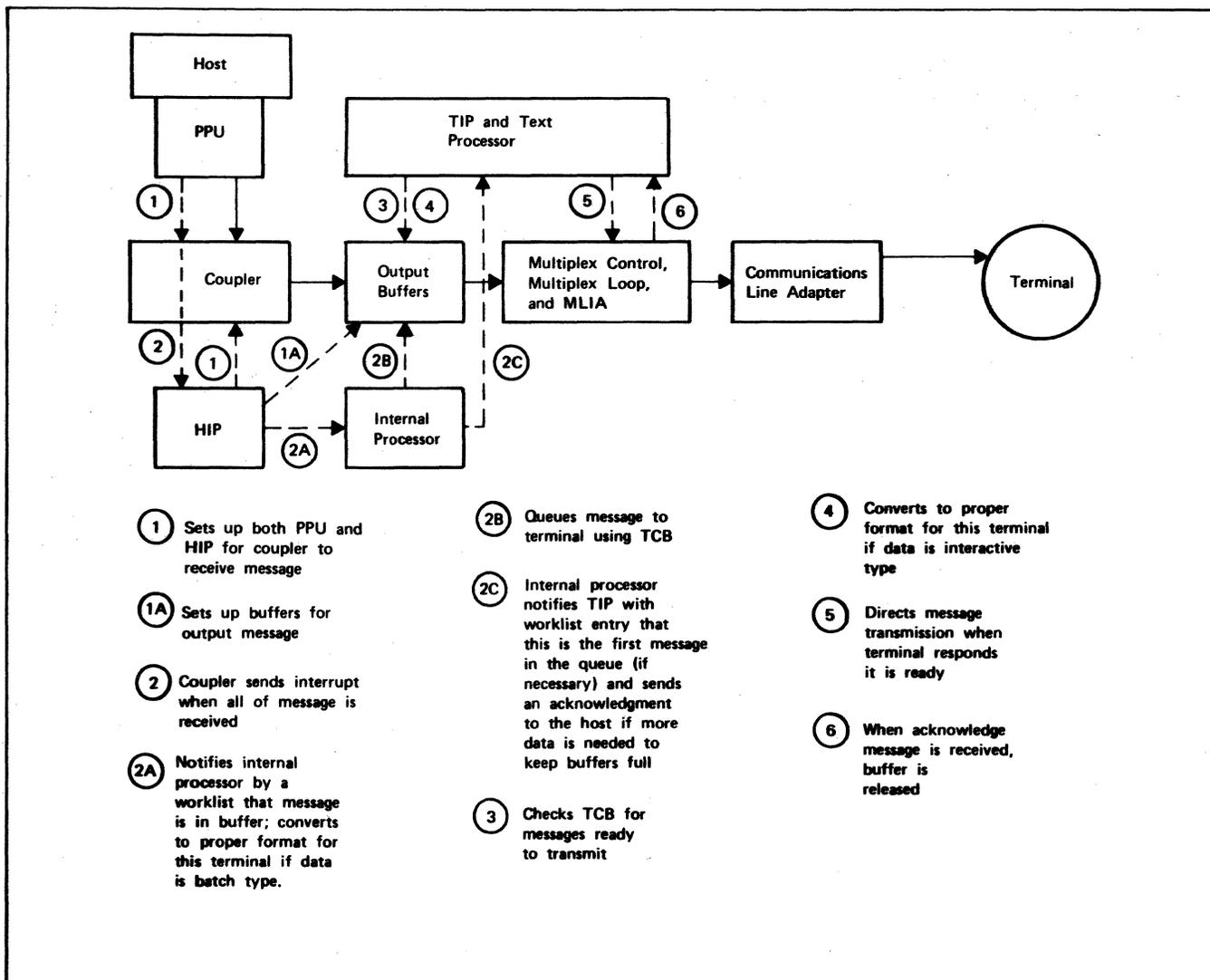
Figure 1-7. Simplified Output Message Processing
