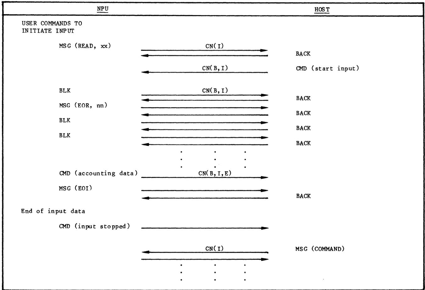
Figure H-2. General Batch Input Flow
