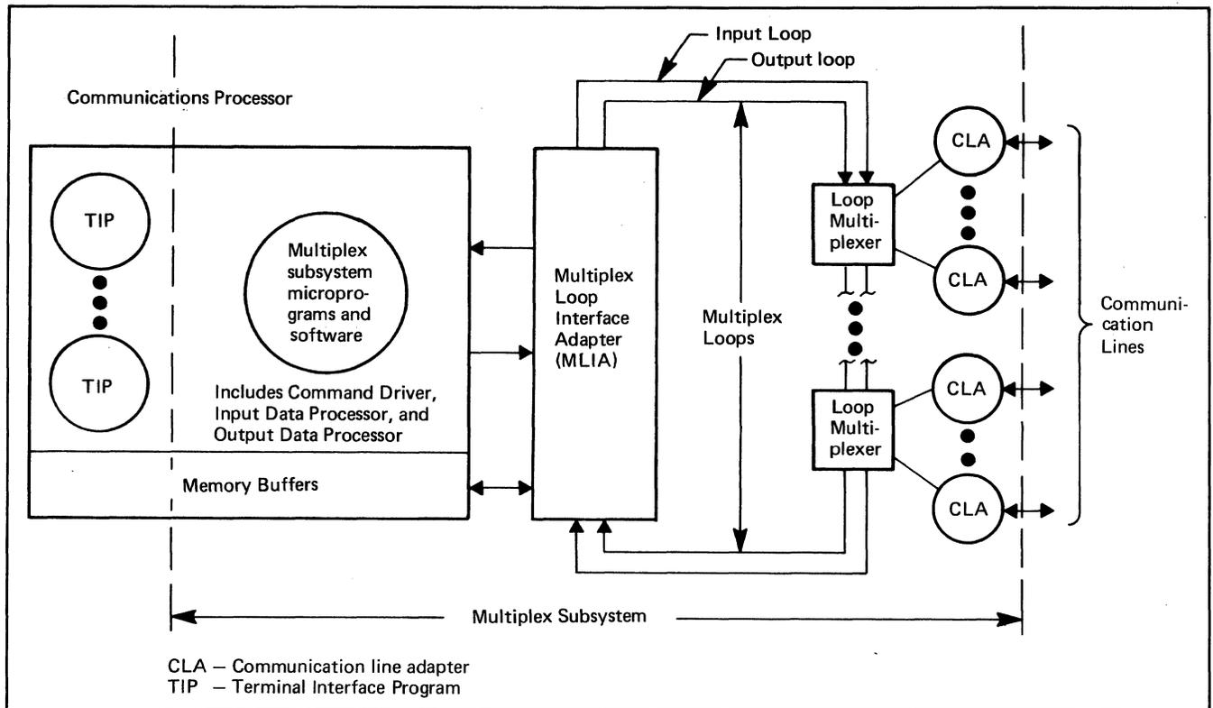
Figure 2-2. Basic Elements of the Multiplex Subsystem
