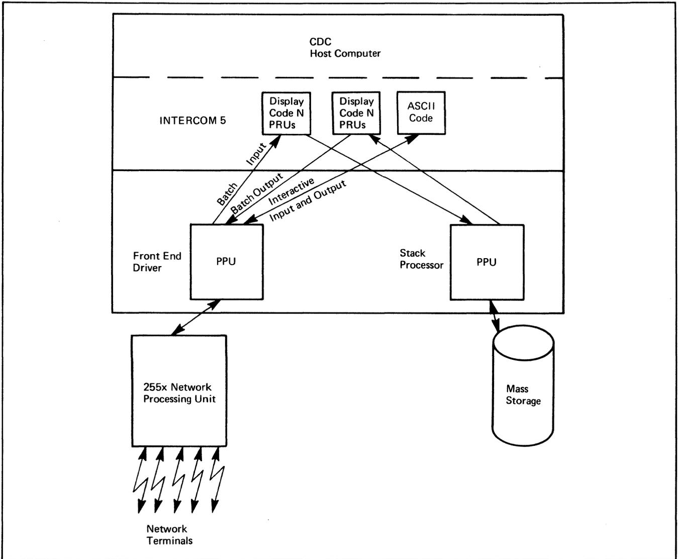
Figure 1-5. INTERCOM and CCI Data Flow
