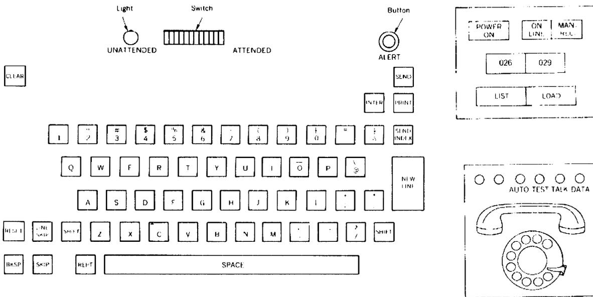
Figure 2-6. Standard 217-13, and 217-14 Display Keyboard (ASCII)
