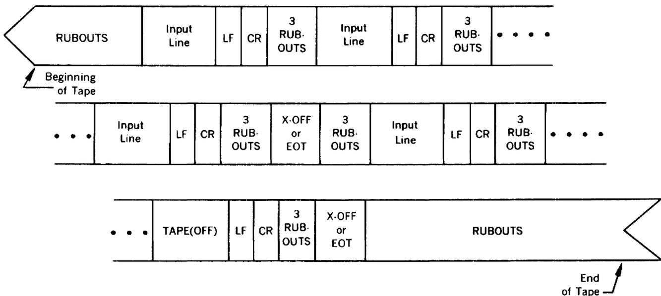
Figure 2-4. Punched Tape Format
