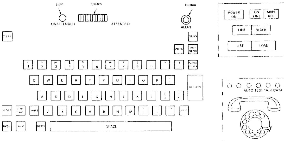
Figure 2-5. Standard 214-11, 214-12, 217-11, and 217-12 Display Keyboard (BCD)
