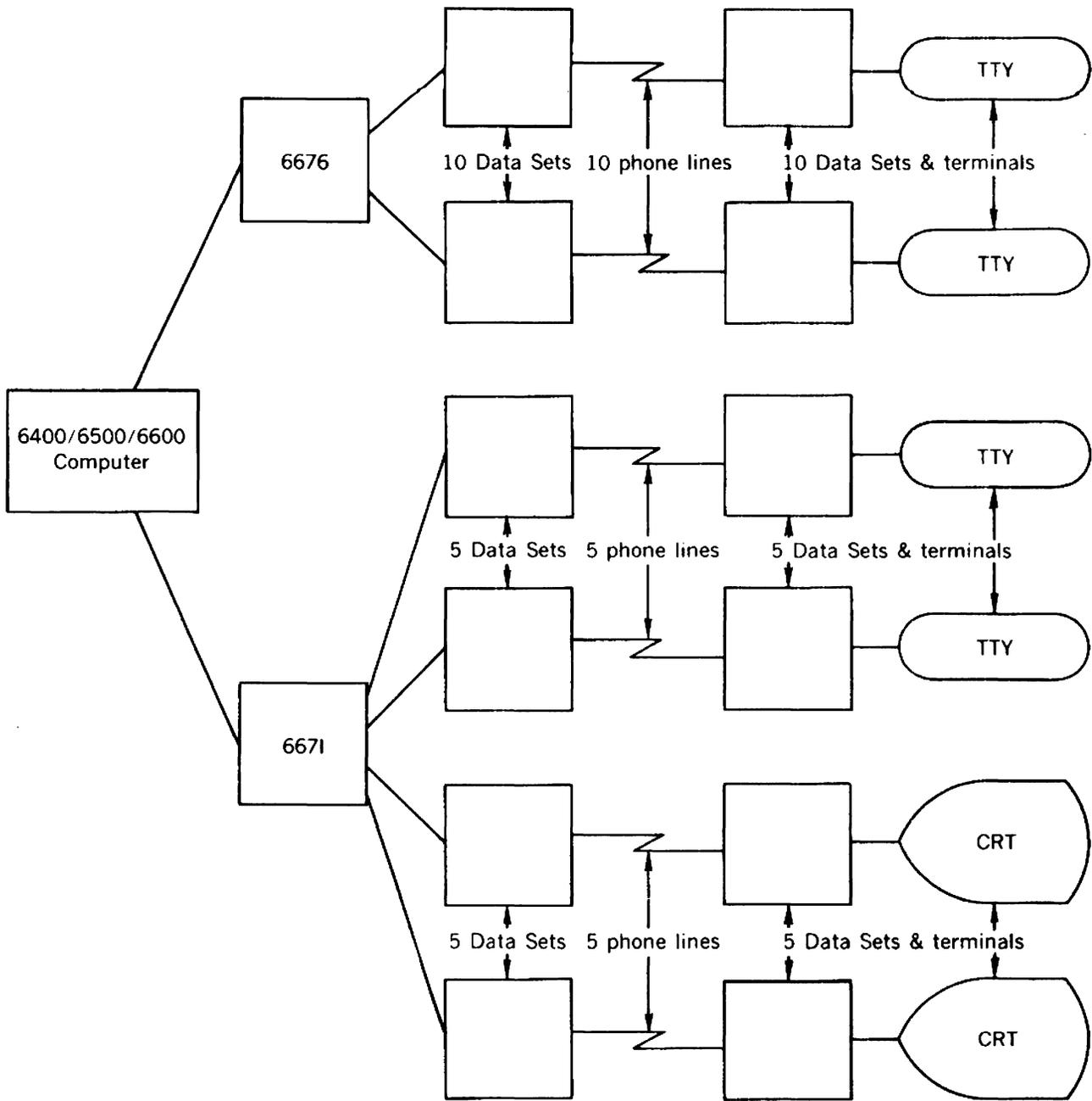
Figure E-1. Mixed Configuration with 5 Display and 15 Teletype Terminals
