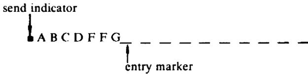
Press BKSP key three times to move entry marker under F:
