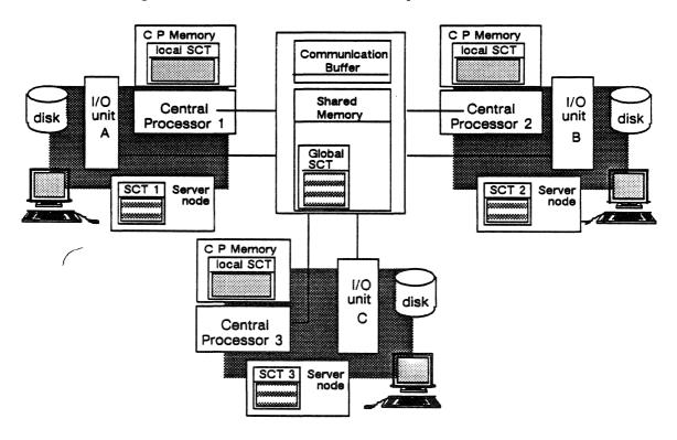
Figure 3-6. Independently functioning central processors.
