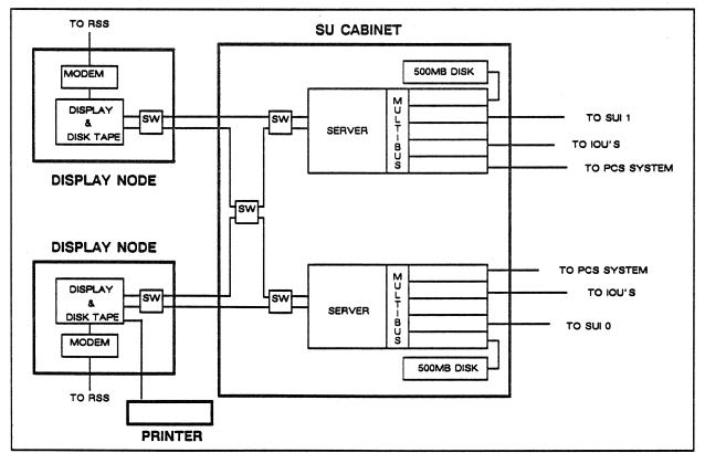
Figure 9-6. Hardware components of the service unit.
