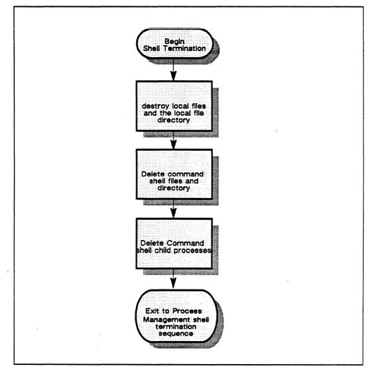
Figure 2-26. Shell Termination flow chart.
