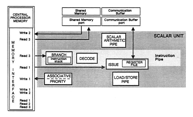
Figure 5-8. The internal components of the scalar processor.
