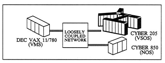
Figure 7-8. DEC VAX 11/780, CYBER 850, and CYBER 205 on an LCN
