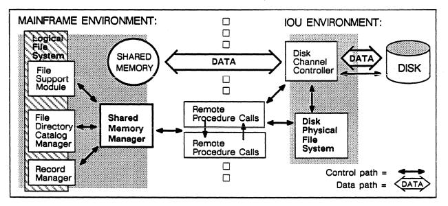
Figure 6-11. Software components involved in file transfers between disk and shared memory.
