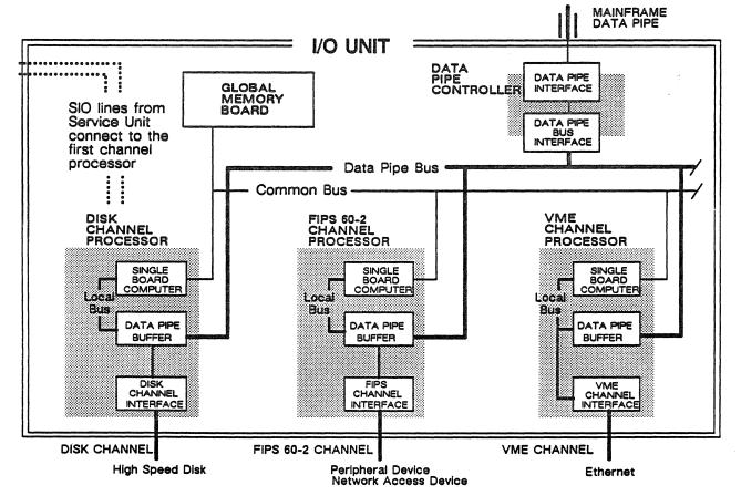
Figure 6-2. Internal components of an I/O unit.
