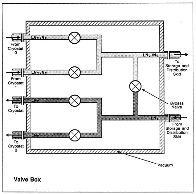
Fig. 10-3. Functional diagram of the valve box operation.
