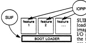
SUIF calls the ROM-resident boot loader to load the IOP initialization images from shared memory to the I/O processor. The boot loads the features in the image and they are then initialized by IOPIP.
