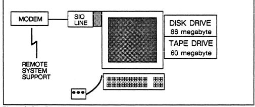
Figure 9-8. Display node components.
