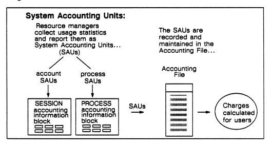
Figure 3-10. How the accounting system collects, stores, and uses SAUs.
