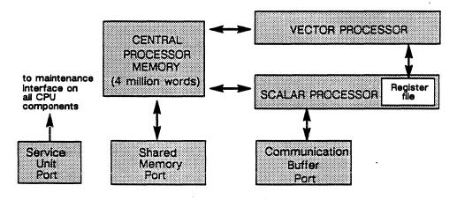
Figure 5-3. Components in the ETA10 central processing unit.
