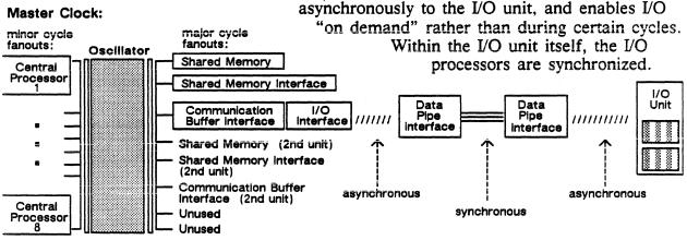
Figure 5-17. System synchronization in the ETA10.
