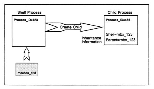
Figure 2-15. The shell creates a process, passing inheritance information.
