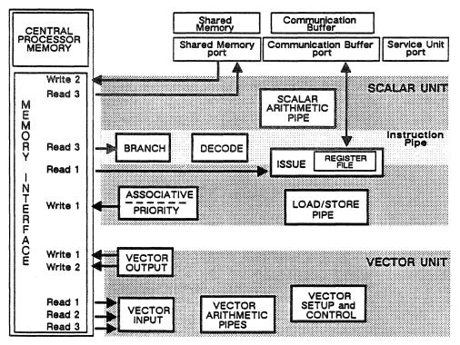
Figure 5-6. Components in the central processor.
