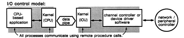
Figure 6-4. Control model for I/O transfers.
