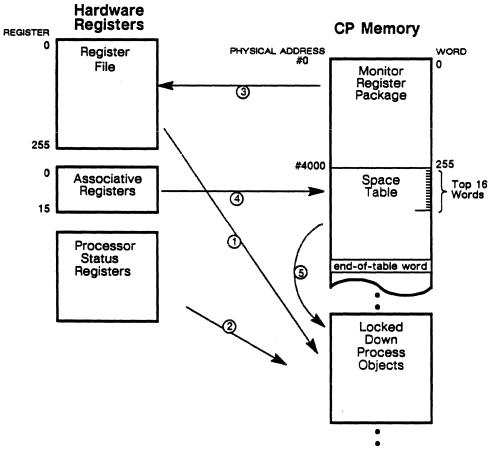
Figure 4-4: Job to Monitor Mode Exchange.
