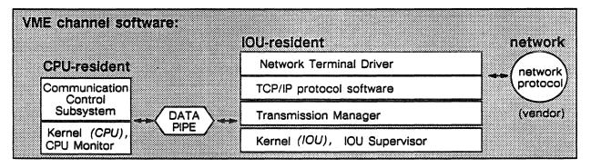
Figure 6-10. VME channel software components with central processor-resident software.
