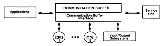
Figure 3-5. Processors/components with access to the communication buffer.
