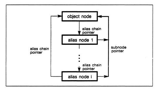
Figure 4-14. An alias chain showing the node pointers.
