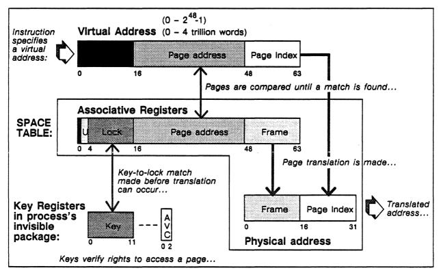
Figure 5-25. Diagram of the virtual-to-physical addressing mechanism.
