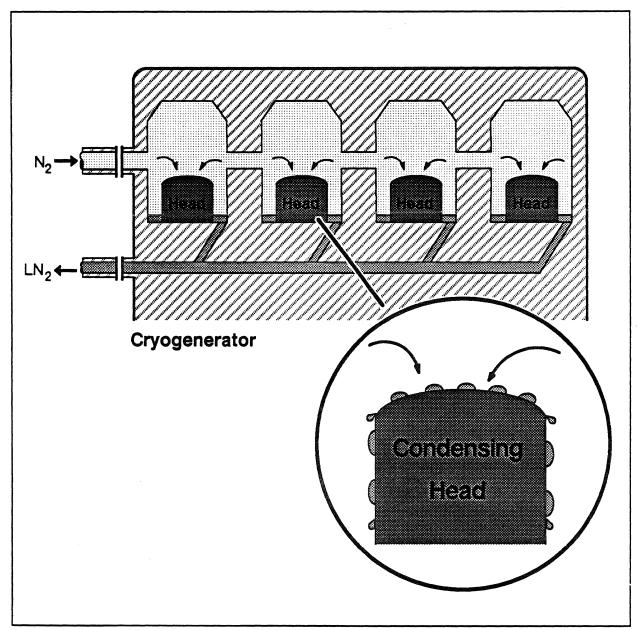
Fig. 10-5. Functional diagram of cryogenerator operation.
