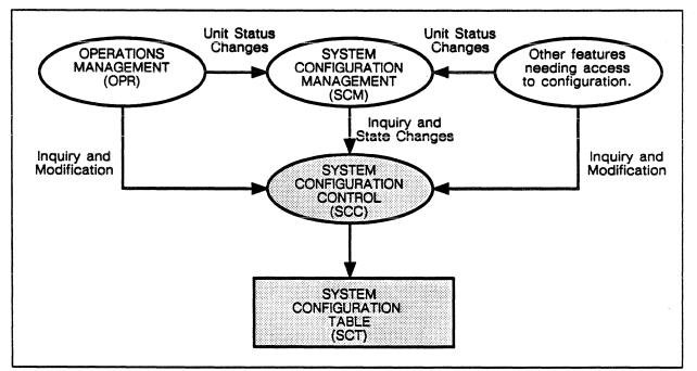
Figure 9-23. System configuration control interfaces with other, features.
