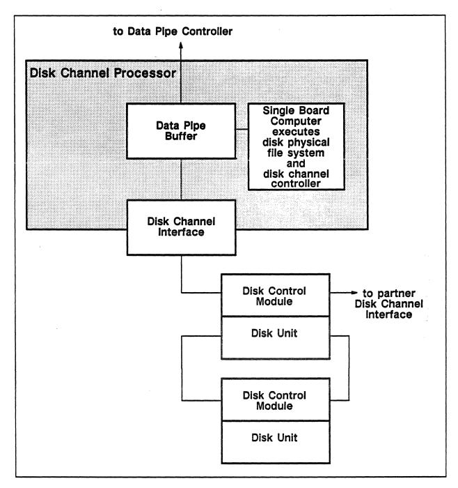
Figure 8-2. Disk channel processor and two disk units.
