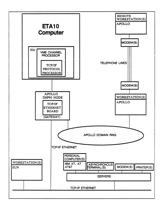
Figure 7-1. Sample Open Interconnection Network connections.
