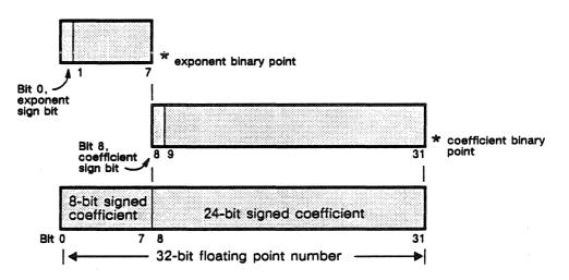
Both coefficient and exponent are expressed as twos complement, signed integers. Numbers are of the form  $c \cdot 2^{\chi}$ , where c is the 24-bit signed coefficient, x is the 8-bit signed exponent, and the base is 2.
