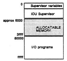
Memory on the single board computer is used for the major components of IOU software and for maintaining some IOU tables. It is also used for channel procesor message passing.
