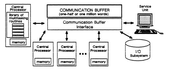
Figure 5-31. Processors/components connecting to the communication buffer.
