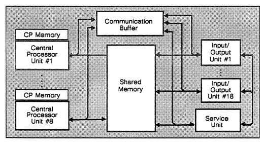
Figure 5-2. Communication paths between the ETA10 mainframe components, the I/O subsystem, and the service unit.
