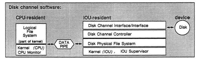
Figure 6-8. Diagram of disk channel – central processor software components.
