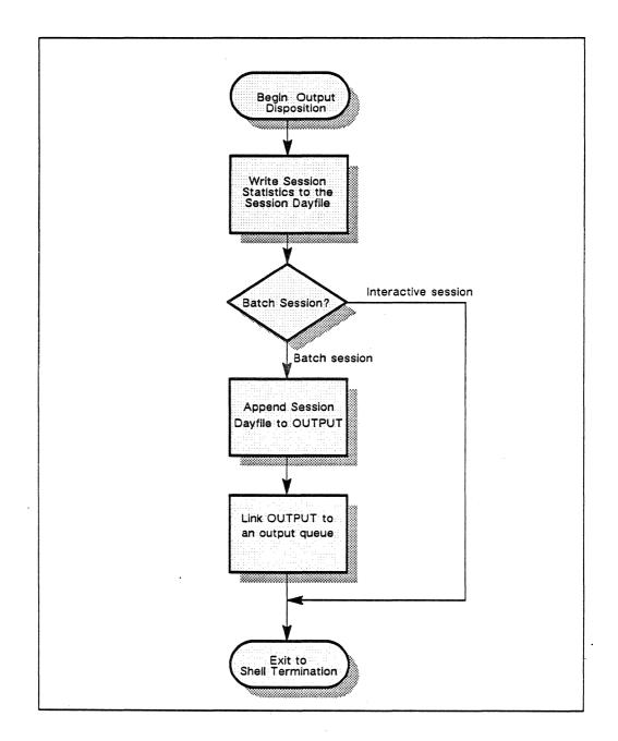
Figure 2-25. Output Disposition flow chart.
