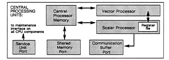
Figure 1-5. Components in the ETA10 central processing unit.
