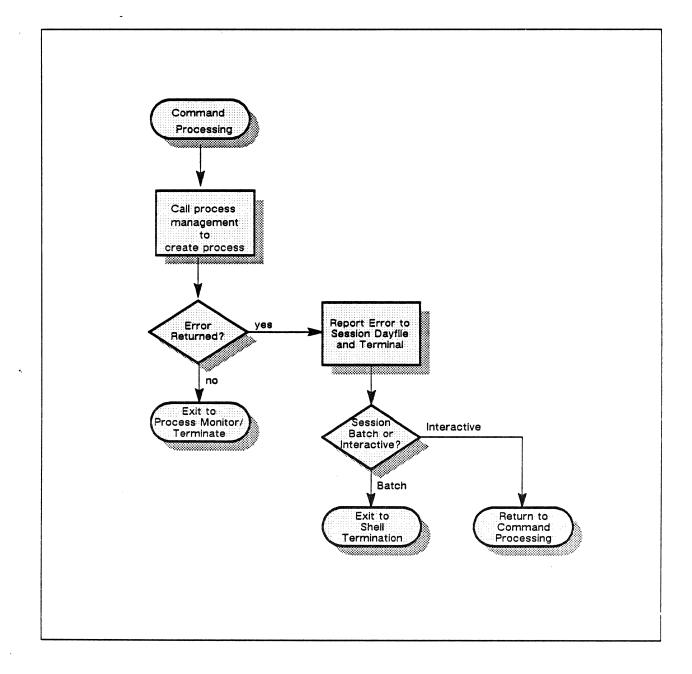
Figure 2-23. Process Create flow chart.
