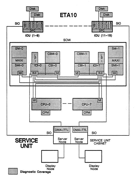
Figure 9-14. Diagnostic coverage of the ETA10 System.
