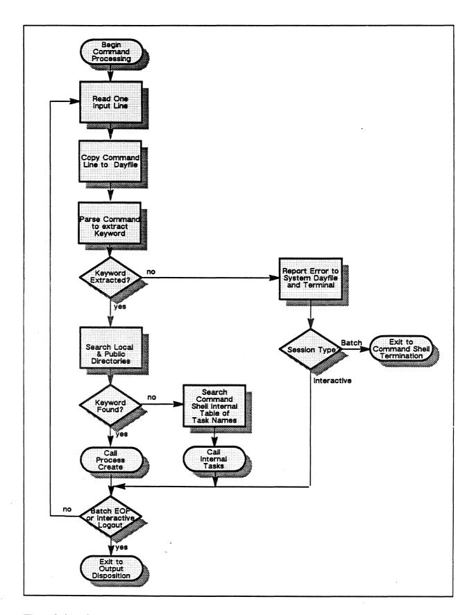
Figure 2-21. Command Processing flow chart.
