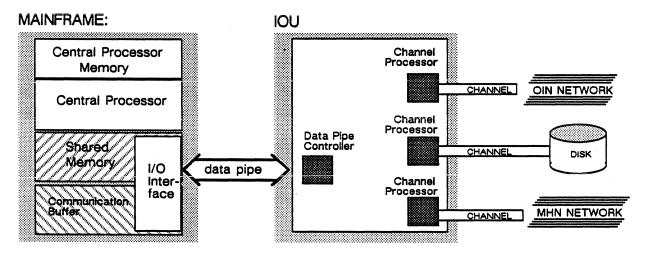
Figure 6-1. The data path between the I/O subsystem and the ETA10 mainframe.
