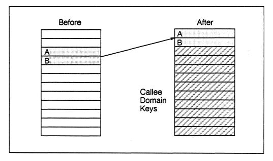
Figure 4-34. Shifting incoming parameter keys to outgoing parameter keys in a forward domain change.
