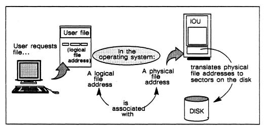
Figure 3-7. I/O file request and address translation process.
