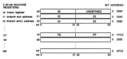
Figure 5–13. Structure of the register file.
