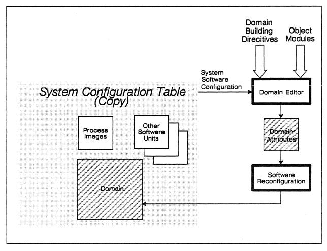
Domain editor and software reconfiguration can also delete inactive versions of a domain, and display information about a domain.
