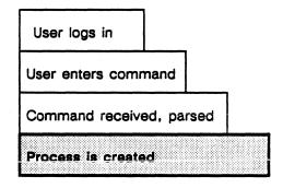
When Process Create is called by the command shell and given the ID of the file to execute, it first assigns a unique process ID to identify that process throughout the system. Inheritance information for the process is retrieved from the command shell, global scheduler, and user management features.
