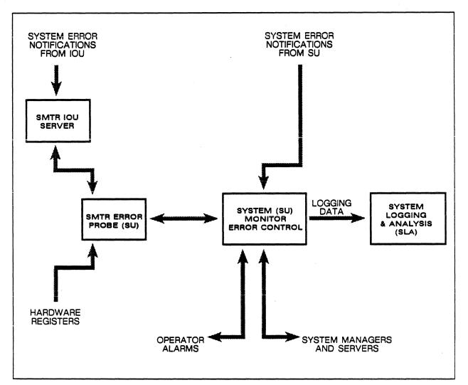
Figure 4-37. Components and interfaces of the system monitor.
