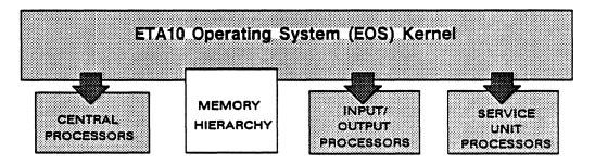
Figure 1-3. The EOS kernel is distributed across system hardware.
