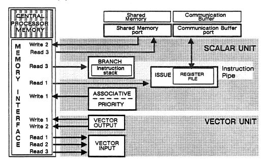
Figure 5-27. Components that read and write to the processor memory interface.
