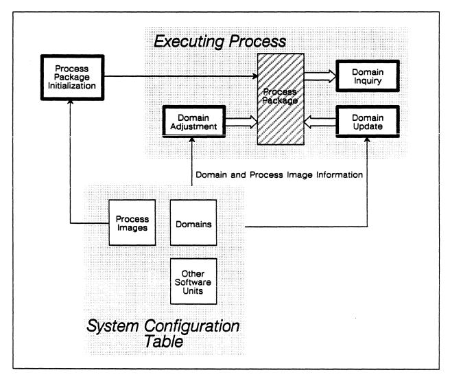
Figure 4–32. The process of process initialization and execution.
