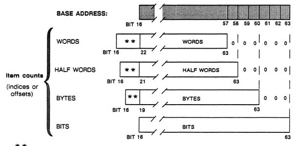
These bits in the index or offset are shifted off and do not enter the address calculation.
