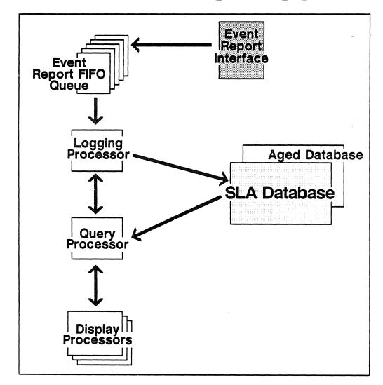
Figure 4-38. SLA Architecture.
