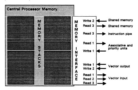
Figure 5-20. Functional diagram of central processor memory.
