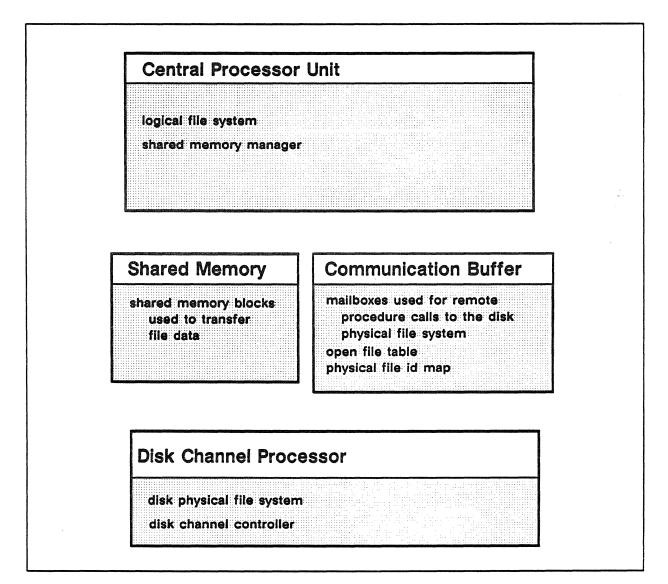
Figure 8-3. Residence of software servicing the disk system.
