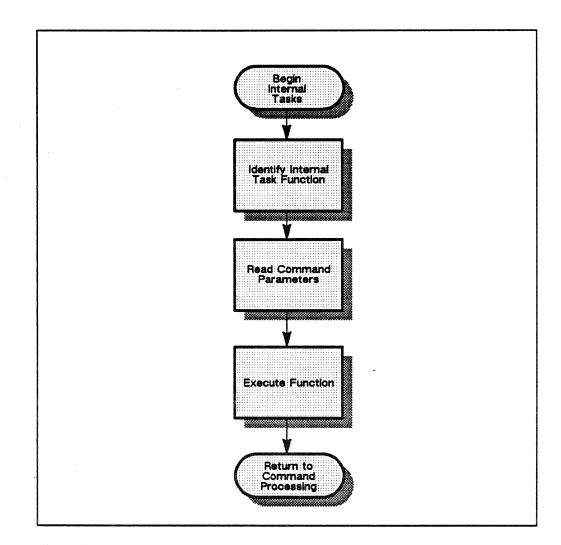
Figure 2-22. Internal Tasks flow chart.
