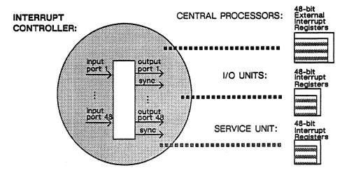
Figure 6-17. The system-wide interrupt network and interrupt controller.
