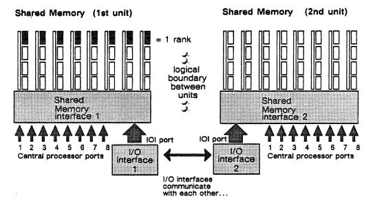
Figure 5-28. Shared memory units in a redundant system.
