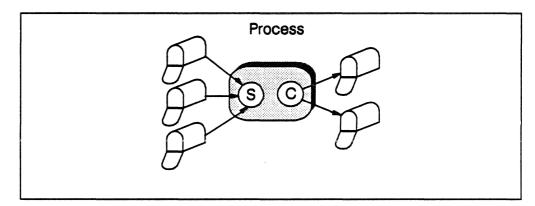
Figure 4-24. A process which is both a client and server to different mailboxes.
