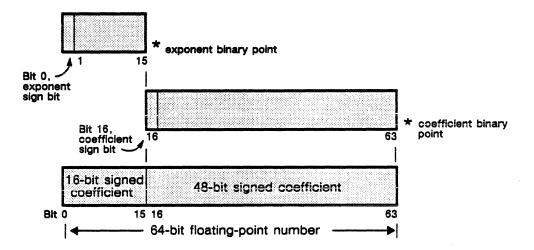
Both coefficient and exponent are expressed as twos complement, signed integers. Numbers are of the form  $c \cdot 2^{X}$ , where c is the 48-bit signed coefficient, x is the 16-bit signed exponent, and the base is 2.
