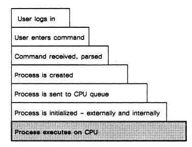
While executing, the process may perform any number of operations, depending on the application. During its execution, the process might retrieve inheritance information from the process descriptor block. The operating system does resource accounting, such as tracking the time spent by the process in the application domain. The process can communicate with other processes on the central processor using IPC mailboxes.
