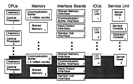
Figure 1-7. Redundancy options in the ETA10 super-cooled systems.
