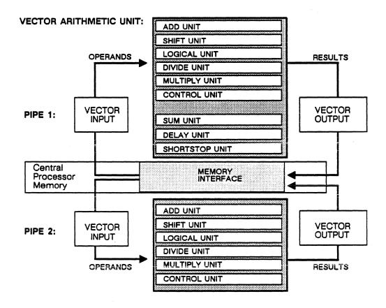
Figure 5-12. Internal components of the vector pipelines.
