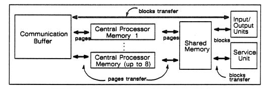
Figure 5-19. Transfer paths between the types of system memories.
