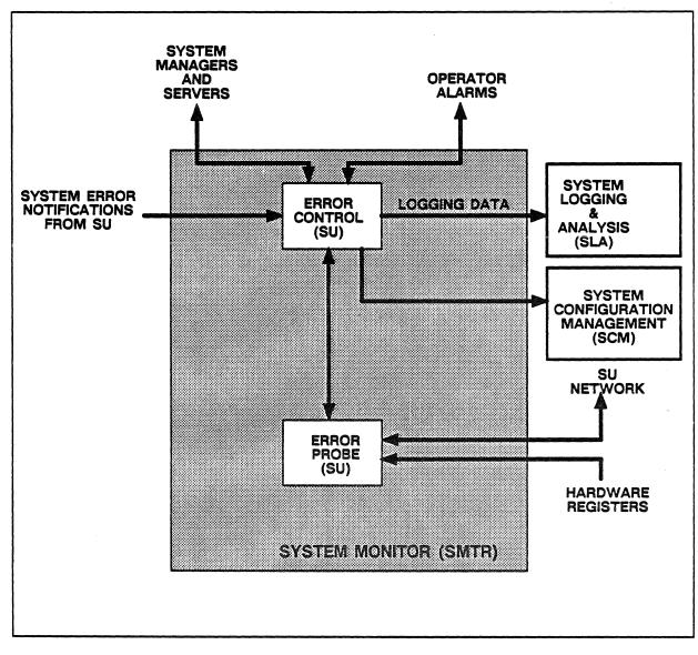
Figure 9-18. System monitor interfaces.
