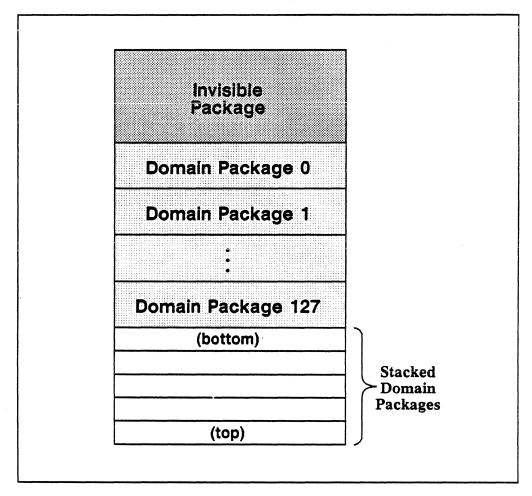
Figure 4-35. Process package structure.
