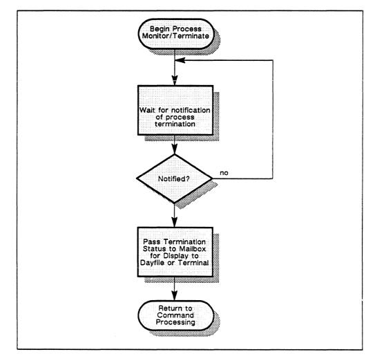
Figure 2-24. Process Monitor/Terminate flow chart.
