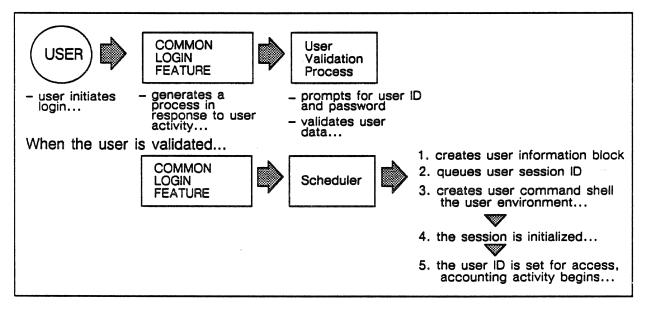
Figure 2-6. Interactive login process involving the common login feature and global scheduler.
