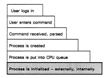
One process management server (PM server) runs on each central processor in an ETA10 system and handles all processes on that processor. When global scheduler calls the PM server to initialize a new process, external and internal initialization take place.
