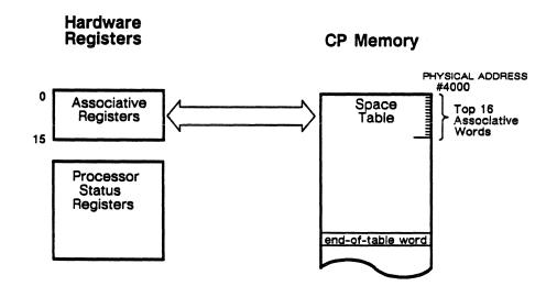
Figure 4-2: Virtual address mechanism.
