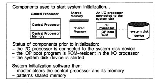
Figure 6-7. Components used in the system installation process.
