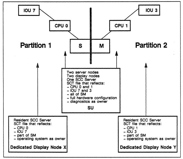
Figure 9-20. System configuration tables on a partitioned system.
