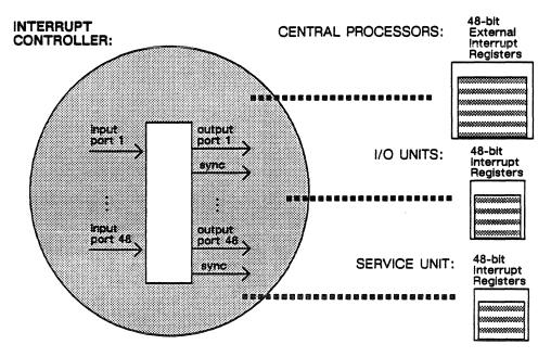
Figure 5-16. The system-wide interrupt network.
