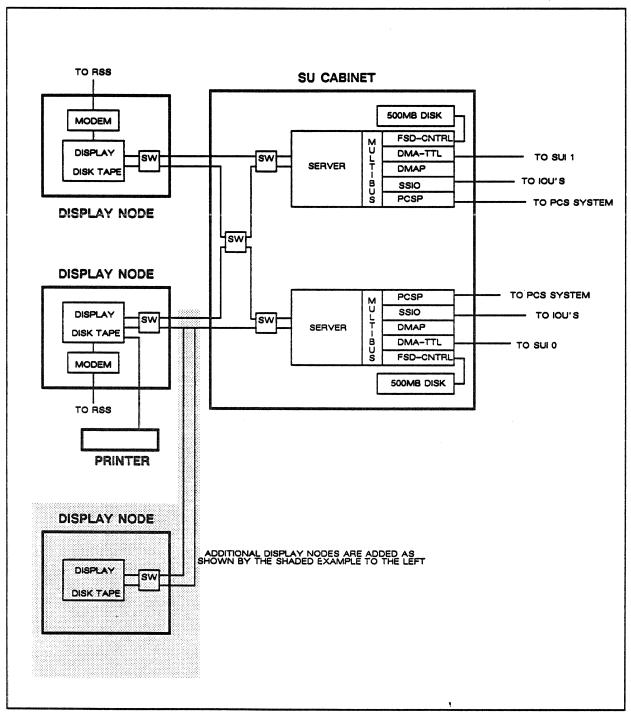
Figure 9-7. Hardware configuration of the SU.
