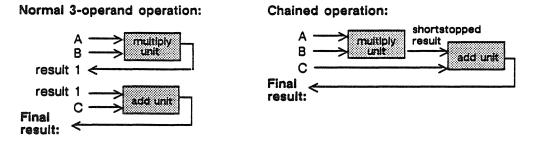
Figure 5-11. Comparison of chained and normal 3-operand operations.
