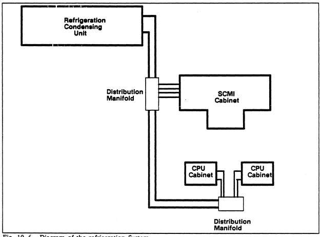
Fig. 10-6. Diagram of the refrigeration System.
