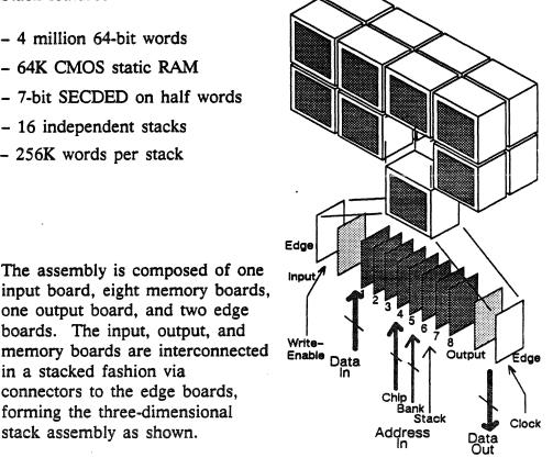
Expanded view of central processor memory stack assembly. Figure 5-21.
