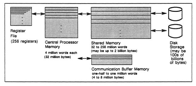
Figure 5-4. Components of the memory hierarchy.
