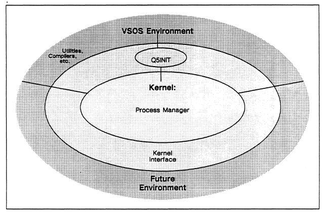
Figure 2-2. Calling a kernel function from an environment.
