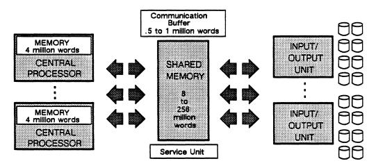
Figure 1-4. System components of the ETA10.
