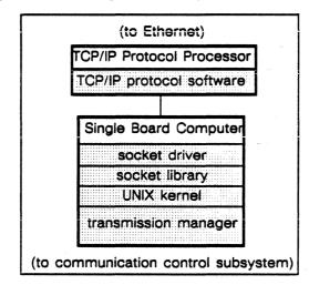
Figure 7-6. TCP/IP protocol software to transmission manager interface
