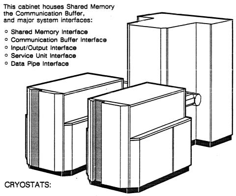
These are special containers that immerse the Central Processors in a liquid nitrogen bath.
