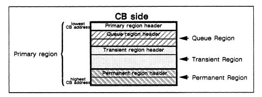
Figure 4-17. A Communication buffer side is typically divided into regions for the three object types.
