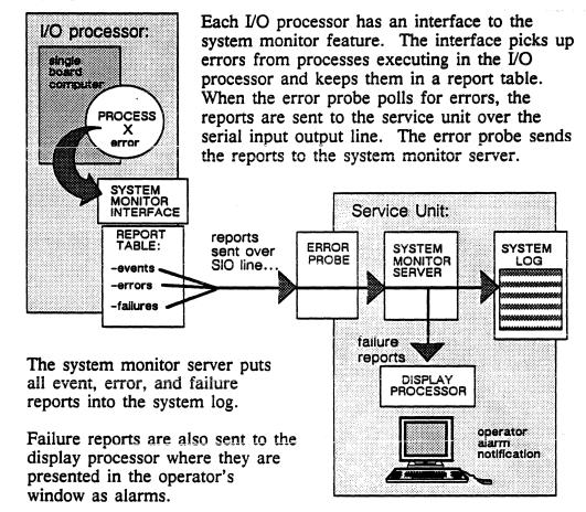
System features attach severity level flags to each report sent to a system monitor interface. When the flag indicates a failure, those reports are recorded and are also processed as operator alarms. An error report might report a disk sector problem or a single error correction-double error detection (SECDED) error. A failure report would indicate a failed disk device or a fatal double SECDED error.
