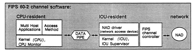
Figure 6-9. FIPS channel software components with central processor-resident software.
