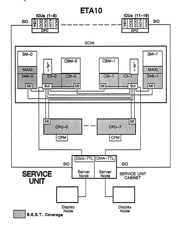
Figure 9-13. B.E.S.T. coverage of the ETA10 System.
