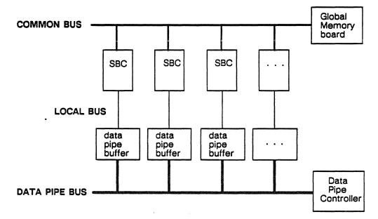
Figure 6–19. The three types of internal IOU buses.
