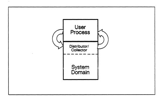
Figure 4-29. Domain protection using a domain distributor/collector.
