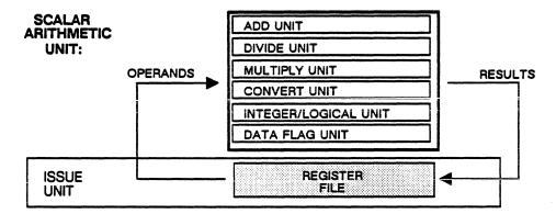
Figure 5–9. The scalar arithmetic unit.
