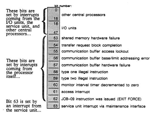
Figure 5-15. Structure of the interrupt register.
