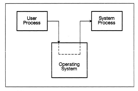
Figure 4-28. Process switch protection mechanism.
