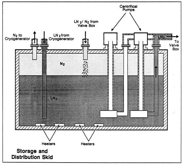
If the cryogenerator is out of service for any reason, an escape valve allows excess gaseous nitrogen to vent from the storage and distribution skid.
