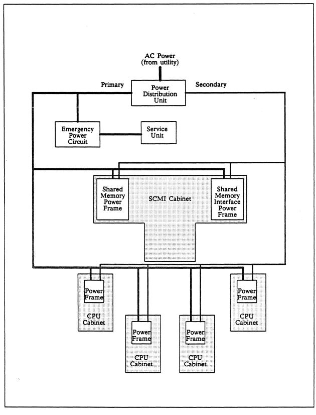
Fig. 10-7. Diagram of power distribution in the ETA10.
