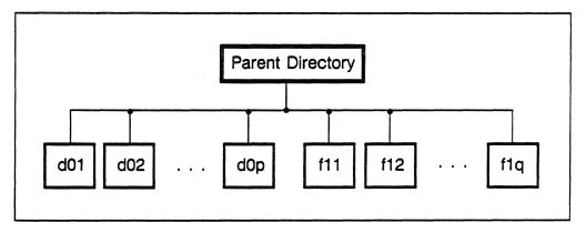
Figure 4-12. A directory structure segment where the d0i represent directories and the f1j represent files.
