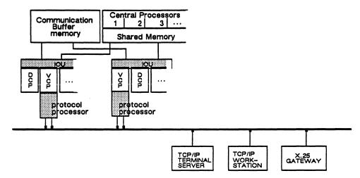
Figure 6-13. Typical attachment of an OIN to the VME channel processor.
