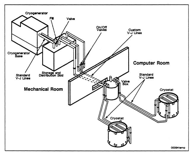
Fig. 10-1. Diagram of the cryogenic system.
