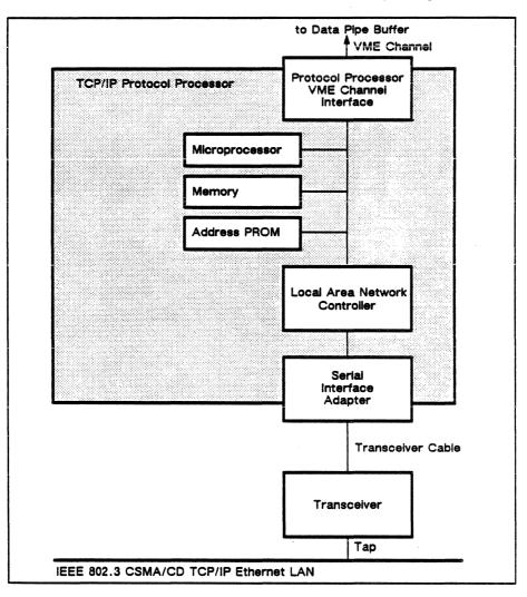
Figure 7-2. TCP/IP protocol processor with its connection to the OIN.
