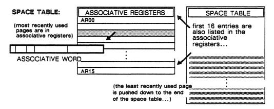
Figure 5-23. Structures in the translation mechanism: associative words, the space table, the 16 associative registers.
