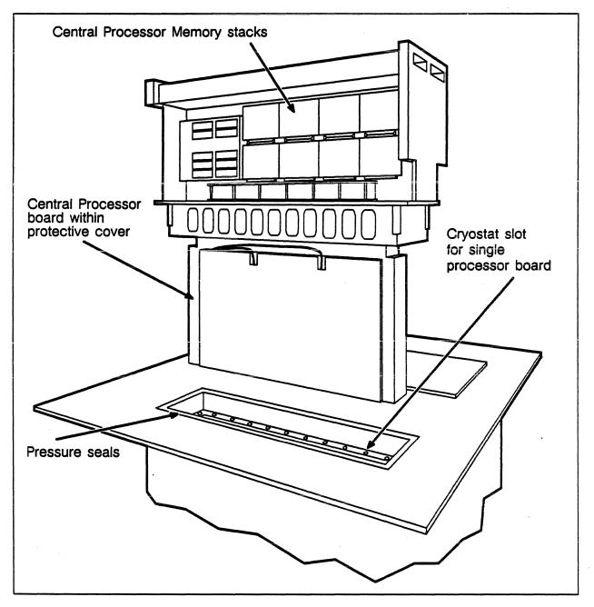
Figure 5-22. Central processor unit assembly for super-cooled operation; boards, interface, memory.
