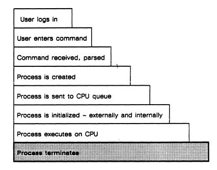
An executing process terminates *normally* or *abnormally*. Normal termination occurs when the process completes its work and issues a process\_terminate call to process management. Process management performs internal and external termination, as described in following paragraphs.
