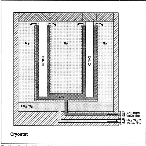
Fig. 10-4. Functional diagram of the cryostat operation.
