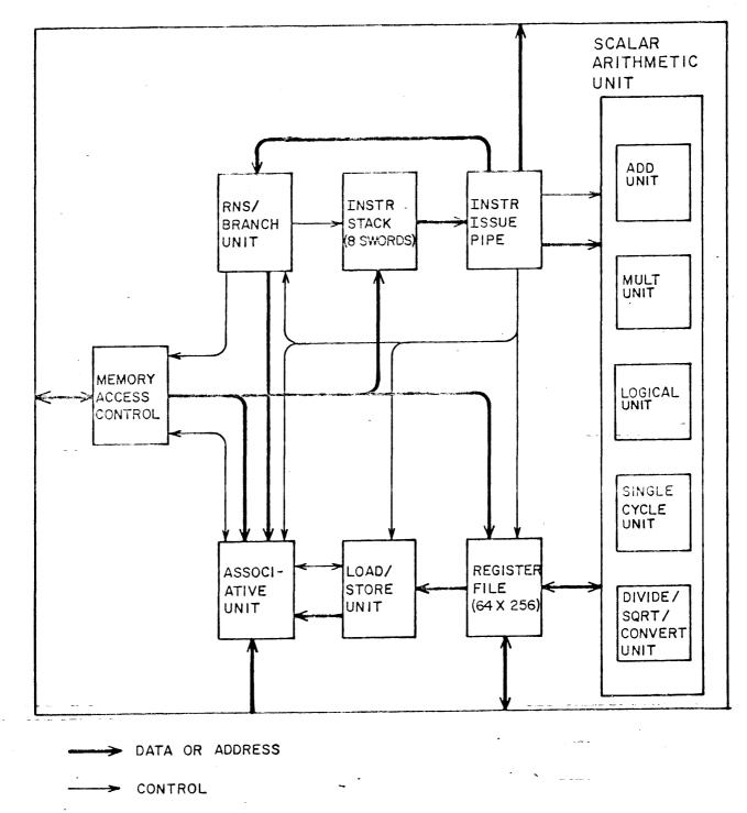
Figure 2-3. LSI Scalar Processor Block Diagram
