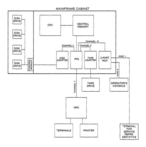
The components are connected to each other through cables and channels. Channels are the paths that connect a peripheral processor to an adapter, a network processing unit, or the 2-port mux.
