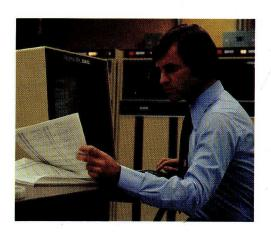
The CDC CYBER 170 series features six compatible computer systems in the mid- to large-scale range. All of these high-performance computers share the same basic architecture: this unique architecture distributes functions among a central processor for computation and auxiliary peripheral processors which perform system input/output and operating system functions.
