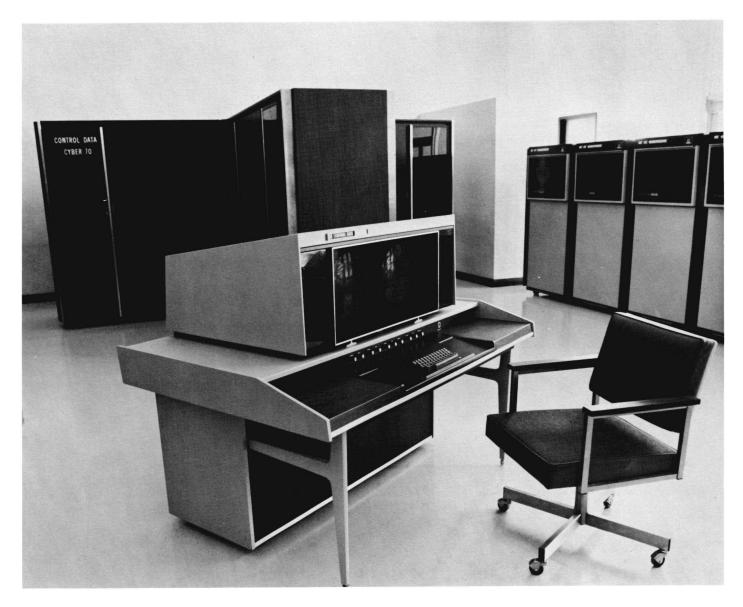
Model 72 is the smallest of Control Data's® CYBER 70 family of compatible computers. This system can be used as a central computer for batch operations and/or as the nucleus for networks of interactive remote terminals. It is suitable in data management, scientific computation, commercial data processing and data communications. Due to hardware and software compatibility among all CYBER 70 systems, Model 72 serves as an expandable base for long-range growth plans.
