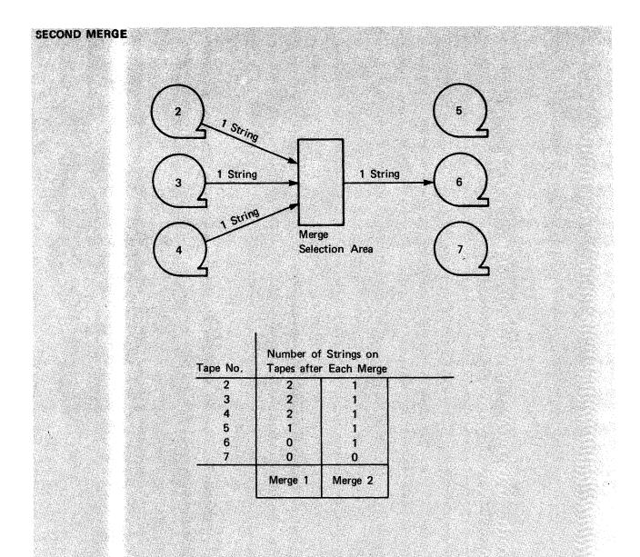
At this point, there is at most one string on each tape. The tapes used as output on the merge pass just completed (5 and 6) are rewound. The tapes used as input (2, 3, and 4), on each of which one string remains to be read, are not rewound, and the final merge phase is entered.
