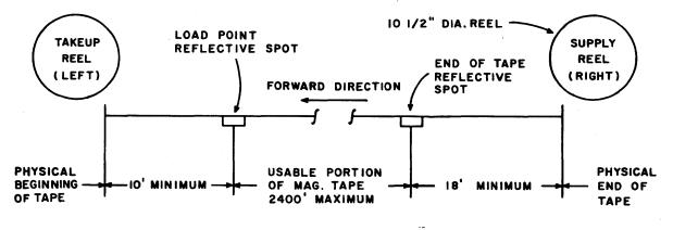
Figure A-2. Physical Layout of Tape
