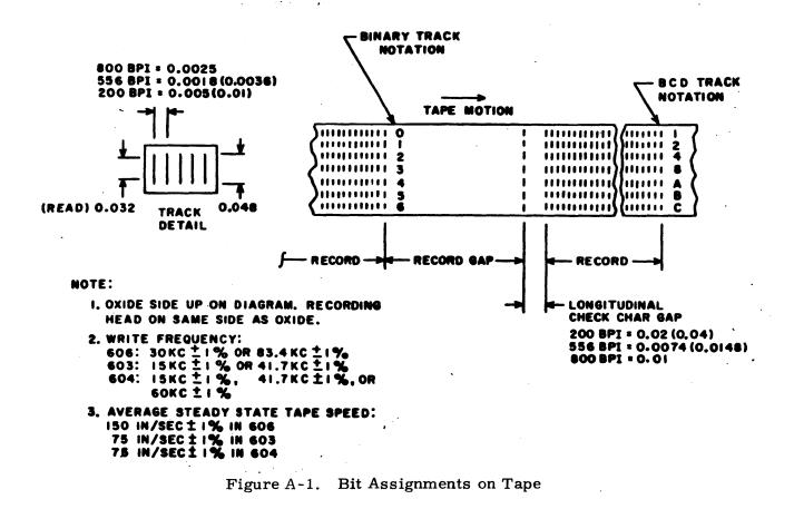
Recorded data on the tape is arranged in groups called records and files. A minimum of one line of information constitutes a record. Adjacent records are separated by a 3/4-inch unrecorded area (record gap). A longitudinal parity bit is recorded in coded\* format at the end of each record; the number of "1's" in each record track is made even.
