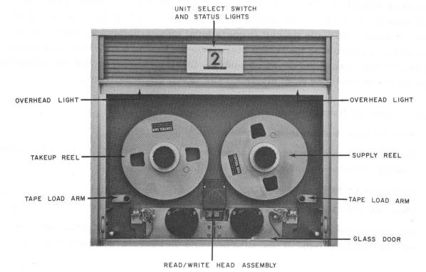
Figure A-4. Tape Load and Unload Mechanics
