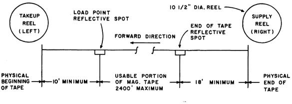
Figure A-2. Physical Layout of Tape
