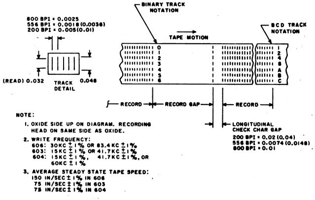
Figure A-1. Bit Assignments on Tape
