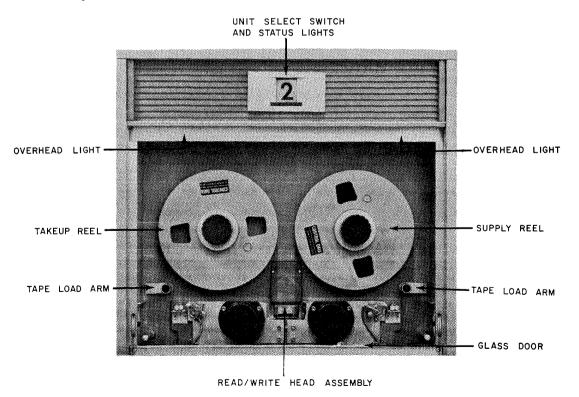
Figure A-4. Tape Load and Unload Mechanics
