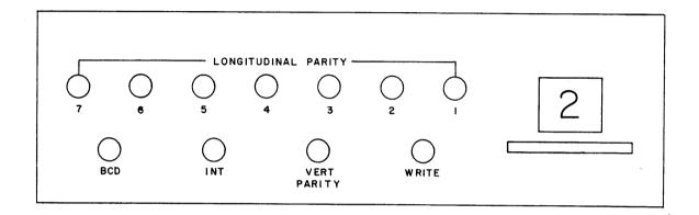
Figure 2. 322X Equipment Number Switch and Indicator Panel\*\*
