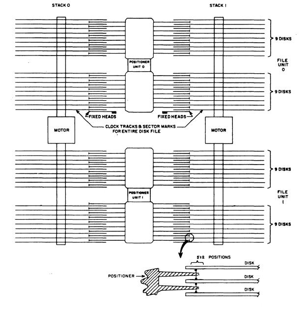
Figure 1-6. 821-2 Disk File Access Mechanism
