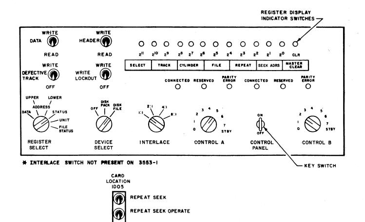
Figure 3-1. Maintenance Panel and Controls
