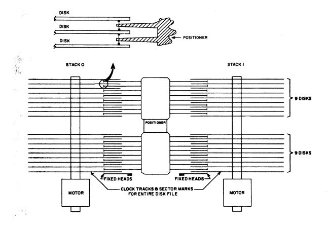
Figure 1-5. 821-1 Disk File Access Mechanism
