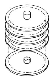
Figure 1-3. Cylinder Concept of Data Recording
