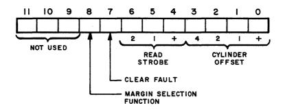
Figure 2-2. Margin Selection Code Bit Assignments
