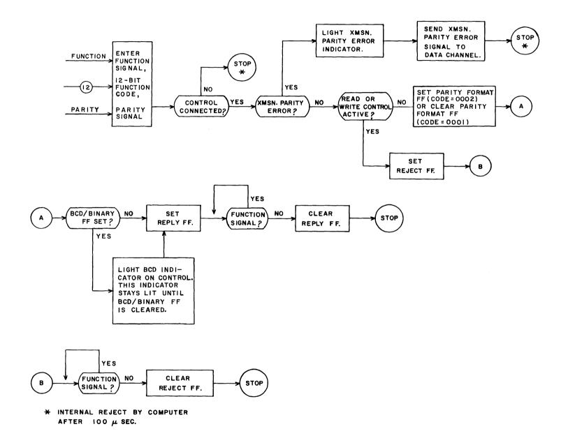
Figure 2-9. Binary Mode Operation
