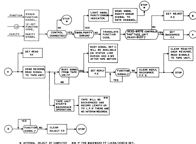
\* INTERNAL REJECT BY COMPUTER  $\times$  IF THE BACKWARD FF (JX38/X39) IS SET, AFTER 100  $\mu$  SEC. TAPE IS MOVED IN A FORWARD DIRECTION.
