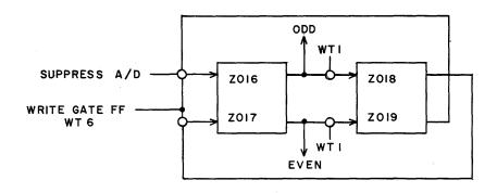
$O_1 \rightarrow B = (WRITE GATE FF) (WT I) (6 - BIT + ODD)$  $O_2 \rightarrow B = (WRITE GATE FF) (WT I) (EVEN) (6 - BIT)$
