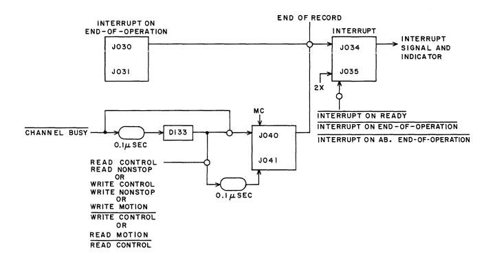
Figure 2-43. Interrupt on End of Operation
