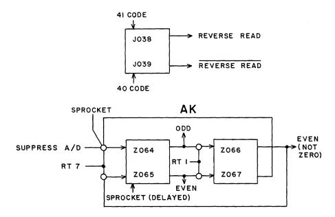
N → X<sub>1</sub> = (REVERSE READ)(EVEN)(RT 2) + (REVERSE READ)(ODD)(RT 2) + (SUPPRESS A/D) N → X<sub>2</sub> = (REVERSE READ)(ODD)(RT 2)(SUPPRESS A/D) + (REVERSE READ)(EVEN)(RT 2) (SUPPRESS A/D)
