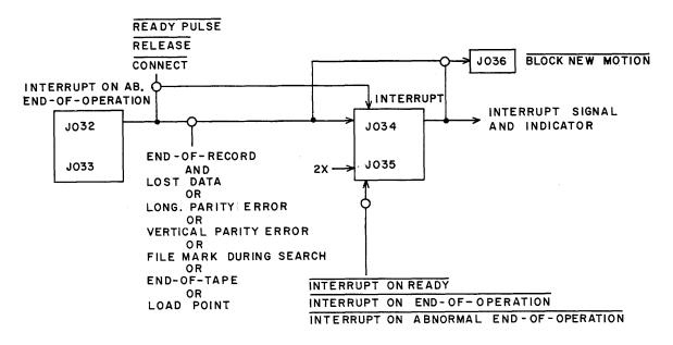
Figure 2-44. Interrupt on Abnormal End of Operation
