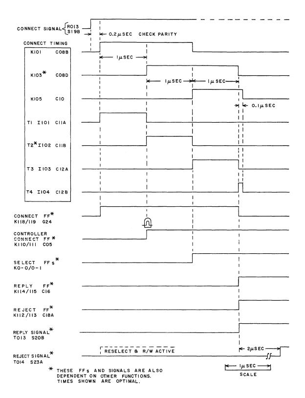
Figure 2-3. Connect Timing
