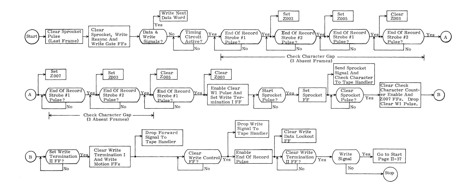
Figure 2-29. Flow Chart: Write Termination
