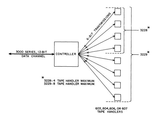
Figure 1-2. 3228/3229 Magnetic Tape System
