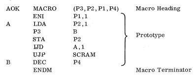
Formal parameter P1 represents an operand, P2 an address, P3 an operation code, and P4 a decimal constant. Locations A and B are local to the macro and may be used elsewhere without ambiguity.
