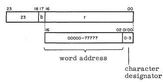
If b = 1, r is modified by index register  $B^2$ ;  $R = r + (B^2)$ . If b = 0, r is not modified (r = R).
