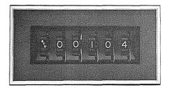
If the WRITE STO switch on the keyboard is depressed and data has been entered into the Communication register, the data is transferred to memory location 00104 when the TRANSFER switch is depressed.
