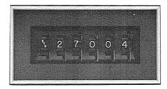
If the READ STO switch on the keyboard is depressed, the contents of memory location 27004 are displayed in the Communication register at a repetition rate determined by the Step Rate control. (If the memory location depicted by the Breakpoint switch exceeds the storage capacity of the system, the computer selects the address that corresponds to the storage capacity of the system.)
