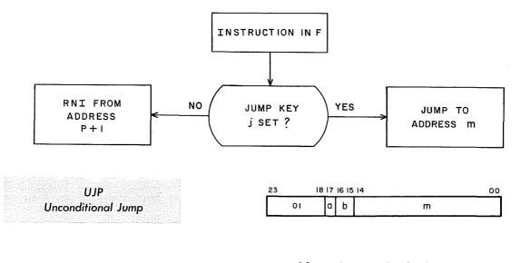
a = addressing mode designator b = index register designator m = storage address; M = m + (B<sup>b</sup>)
