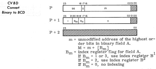
Bits 02-14 of the index register are used for word address indexing (13 bit index-sign extended). Bits 00 and 01 must be set to "1's".
