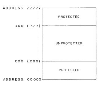
Bxx = 6 switches to select upper area address boundary, lower 9 bits of which are always  $^{\prime\prime}1^{\prime}s^{\prime\prime}$
