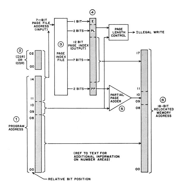
Figure E-1. Address Relocation Process
