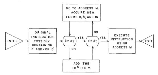
Figure 5-4. Indexing and Indirect Addressing Routine Flow Chart
