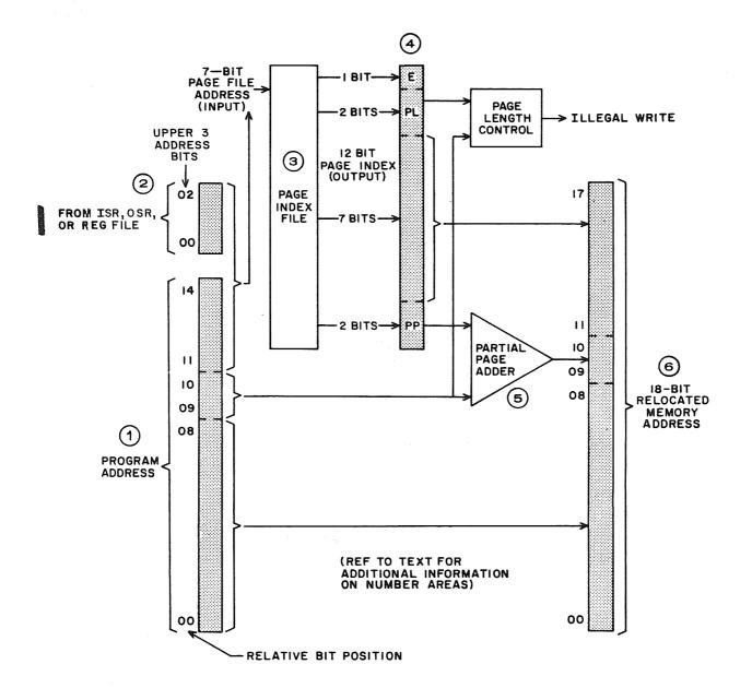
Figure 8-1. Address Relocation Process
