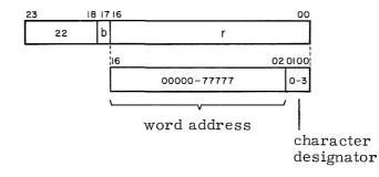
If b = 1, r is modified by index register  $B^1$ ;  $R = r + (B^1)$ . If b = 0, r is not modified (r = R).
