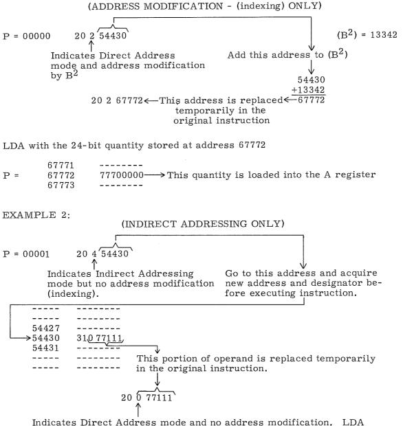
Indicates Direct Address mode and no address modification. LDA with the 24-bit operand stored at address 77111. (If this digit would have indicated additional indirect addressing and/or address modification this must be done before the LDA instruction is executed.)
