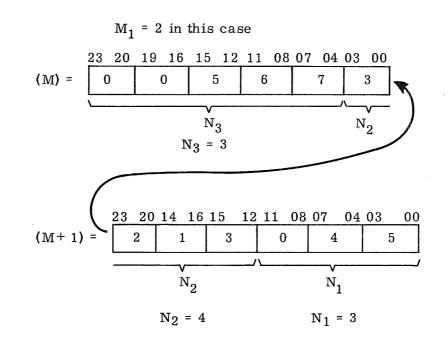
Data words are divided into six 4-bit groups internally by the CPU and are shown here only to illustrate the parameters necessary for determining the instruction execution time.
