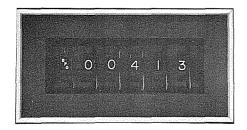
The computer stops only when an attempt is made to read or store an operand at address 00413.
