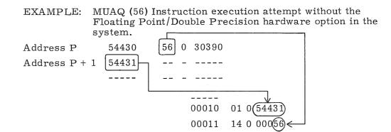
At this point the MUAQ operation may be simulated by software and re-entry to the main program is possible by a jump to the contents of address 00010.
