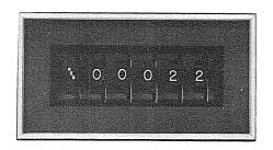
If the READ STO switch on the keyboard is depressed, the contents of register 22 are displayed in the Communication register at a repetition rate determined by the Step Rate control. (Only the lower two digits are of consequence when the REG designator is displayed. In this case register 22, the real time clock, is being referenced.)
