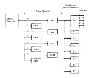
A maximum configuration of data channels. A smaller configuration may be obtained by removing the channels in pairs of odd and even. Any 3307 may be replaced by a 3306, but not vice versa.
