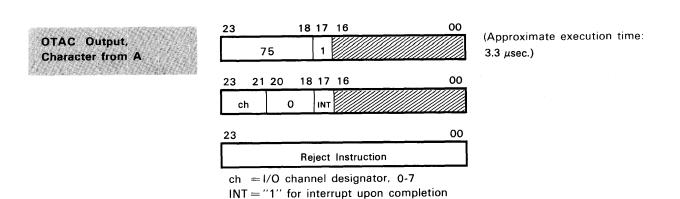
Instruction Description: This instruction transfers a character from the lower 6 bits of A to an external equipment. The original contents of A are retained.
