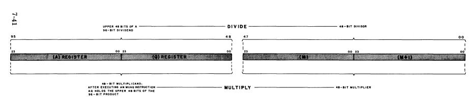
Figure 7-4. Operand Formats and Bit Allocations for MUAQ and DVAQ Instructions
