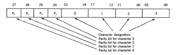
Figure 1-6. Parity Bit Assignments
