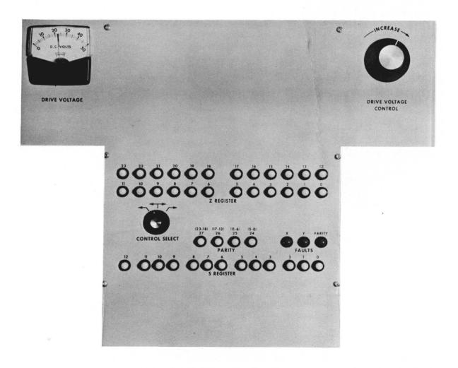
Figure 2-1. Storage Module Control Panel
