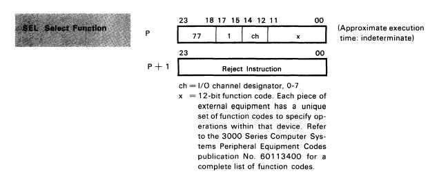
Instruction Description: This instruction sends a 12-bit function code along with a function enable to the unit connected to I/O channel ch. If a Reply is received from the unit within  $100\,\mu\text{sec}$ , the next instruction is read from P+2. If a Reject is received or there is no response within  $100\,\mu\text{sec}$ , a reject instruction is read from address P+1. If the I/O channel is busy, a reject instruction is read from address P+1.
