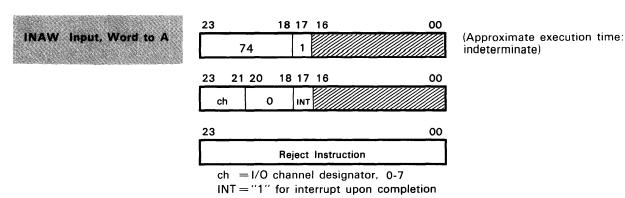
Instruction Description: This instruction transfers a 12-bit byte into the lower 12 bits of A or a 24-bit word into all of A from an external equipment. Transferring 12 or 24 bits depends upon whether a 3206 or 3207 I/O channel is used. (A) is cleared prior to loading and, in the case of a 12-bit input, the upper 12 bits remain cleared.
