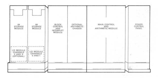
Figure 1-1. Typical 3200 Modular Configuration
