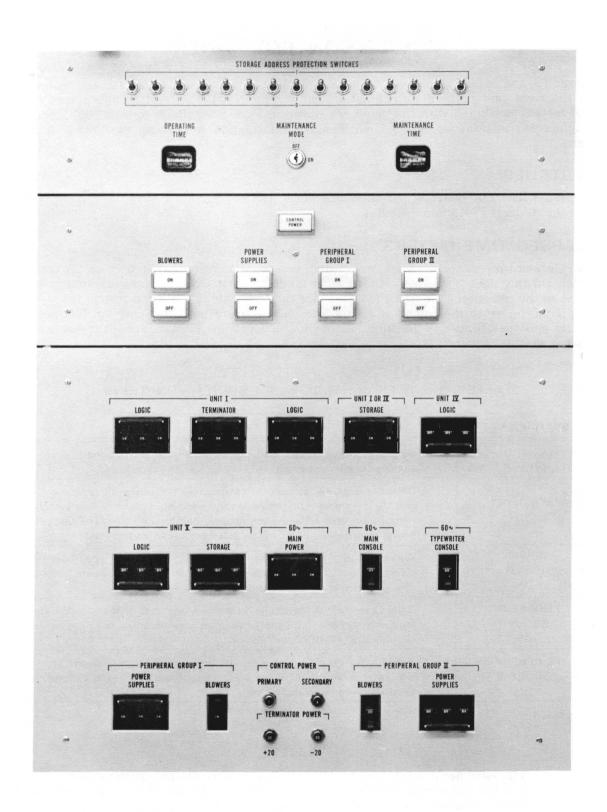
Figure 5-9. Power Control Panel
