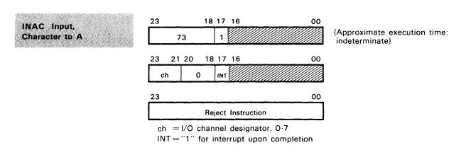
Instruction Description: This instruction transfers a 6-bit character from an external equipment into the lower six bits of the A register. A is cleared prior to loading, and the upper 18 bits remain cleared.
