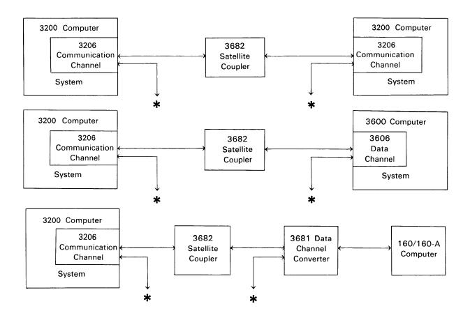
Figure 3-2. Satellite Configurations
