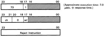
ch = I/O channel designator, 0-3 INT = "1" for interrupt upon completion
