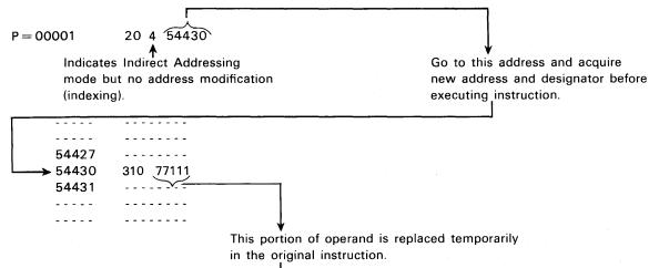
Indicates Direct Address mode and no address modification. LDA with the 24-bit operand stored at address 77111. (If this digit would have indicated additional indirect addressing and/or address modification this must be done before the LDA instruction is executed.)
