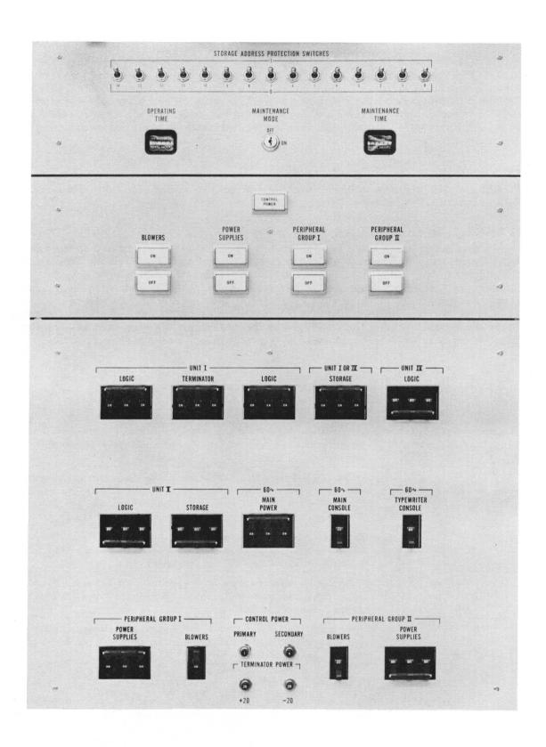
Figure 5-9. Power Control Panel
