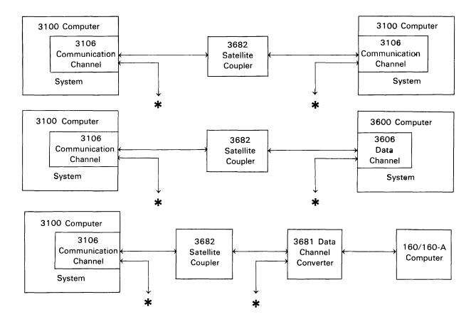
Figure 3-2. Satellite Configurations
