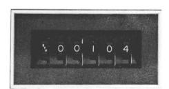
If the WRITE STO switch on the keyboard switch is depressed and data has been entered into the Communication register, the data is transferred to memory location 00104 when the Transfer switch is depressed.
