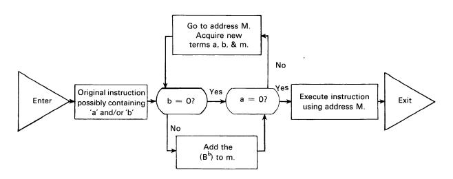
Figure 7-3. Indexing and Indirect Addressing Routine Flow Chart
