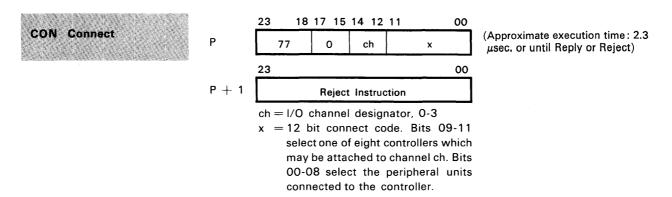
Instruction Description: This instruction sends a 12-bit connect code along with a connect enable to an external equipment controller on I/O channel ch. If a Reply is received from the controller within 100  $\mu$ sec, the next instruction is read from address P + 2. If a Reject is received or there is no response within  $100\mu$ sec, a reject instruction is read from address P + 1. If the I/O channel is busy, a reject instruction is read from address P + 1.
