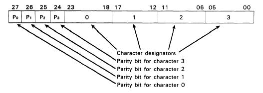
Figure 1-6. Parity Bit Assignments
