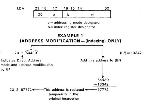
LDA with the 24-bit quantity stored at address 67772
