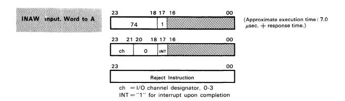
Instruction Description: This instruction transfers a 12-bit byte into the lower 12 bits of A or a 24-bit word into all of A from an external equipment. Transferring 12 or 24 bits depends upon whether a 3106 or 3107 I/O channel is used. (A) is cleared prior to loading and, in the case of a 12-bit input, the upper 12 bits remain cleared.
