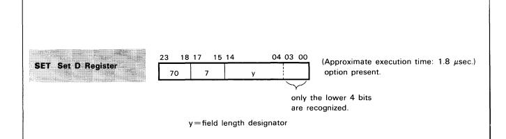
Instruction Description: Load the lower 4 bits of y into the 4-bit D register.
