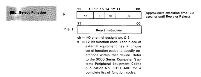
Instruction Description: This instruction sends a 12-bit function code along with a function enable to the unit connected to I/O channel ch. If a Reply is received from the unit within  $100 \,\mu\text{sec}$ , the next instruction is read from P+2. If a Reject is received or there is no response within  $100 \,\mu\text{sec}$ , a reject instruction is read from address P+1. If the I/O channel is busy, a reject instruction is read from address P+1.
