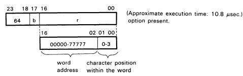
If b = 1, r is modified by (B1); R = r + (B1). If b = 0, r is the unmodified direct address.
