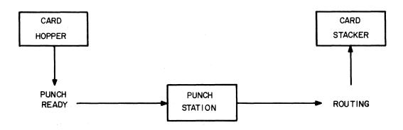
Figure 2. Card Punch Functional Stations
