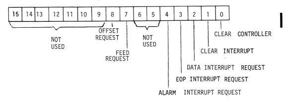
Figure 4. A-Register, Director Function Clear and Interrupt selections may be requested simultaneously or individually. Clears (Controller and Interrupt) will be honored first, but are subordinate to requests that are executed later in the Director Function cycle.
