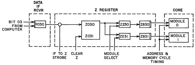
Figure 4. Core Write - Bit 03 Logic Circuit
