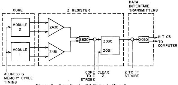
Figure 6. Core Read - Bit 03 Logic Circuit
