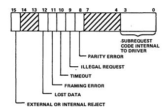
If an error occurs, it is reported by the alternate device handler, and logged in the engineering file. Fault code values are as follows:
