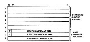
The first added words (words 6 and 7) are necessary to specify the disk address.
