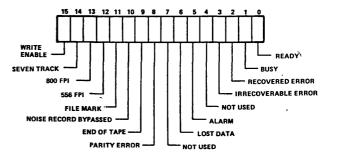
This is not the actual hardware status but is a composed status formed by the driver module called FORMIT based on the information supplied by the hardware status and word 24 (unit/mode) in the physical device table.
