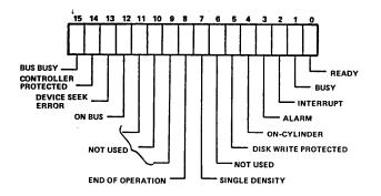
The following errors are detected by the driver:
