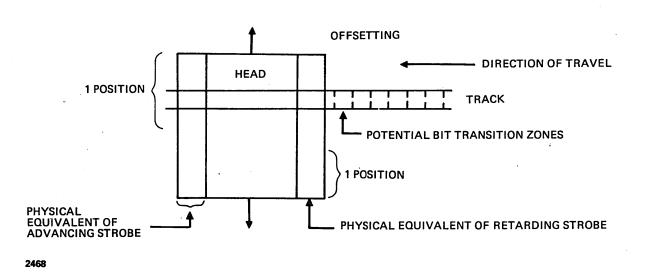
Figure 4-2. Head Positioning
