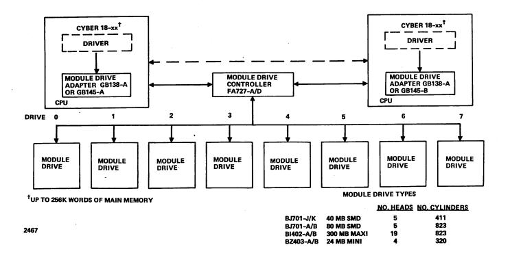
Figure 4-1. Module Drive Driver Maximum Hardware Configuration
