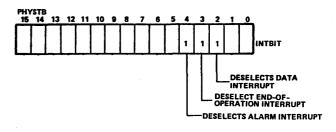
If any INTBIT is set, WAITAD (word 34) must contain the absolute address of the status routine that checks completion of the I/O event. The kernel driver executes the routine and receives control after execution at the continuator entrance of the driver. Transfers are made in ADT mode.
