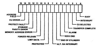
The following hardware statuses can be found in the physical device table assigned to a failed device. Note that the values in the table do not always reflect current status.
