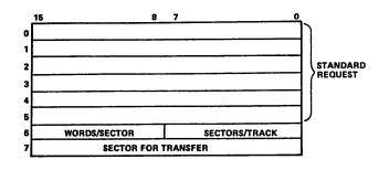
The n parameter determines the number of words to transfer. If n is not a divisor of a sector on an FWRITE request, the data is transferred to the following sector and the balance of that sector is zero filled. On a FREAD request, only the specified number of words is transferred; this in effect masks out the remainder of the last sector.
