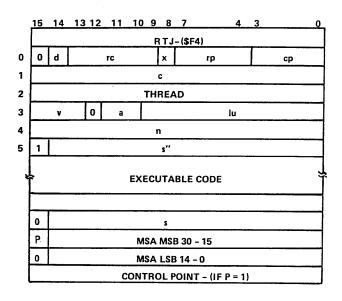
The second request format adds two words that contain mass storage address in line with the conventional data transfer format and that are identified by a direct reference to s (bit 15 equals 0).
