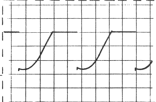
E OUTPUT OF POWER BRIDGE HORIZONTAL 2 MS / CM VERTICAL 20 V / CM
