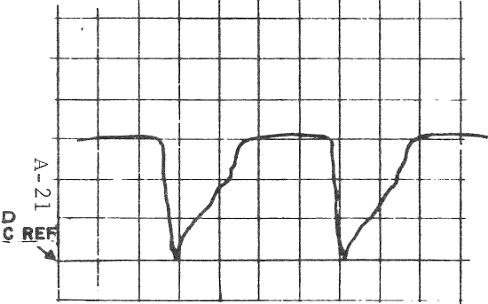
B INPUT TO UNIJUNCTION JUNCTION R16&R17 TO GND HORIZONTAL 2 MS / CM VERTICAL 10V / CM
