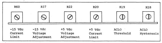
Figure 5-1. Regulator Board Adjustment Potentiometers
