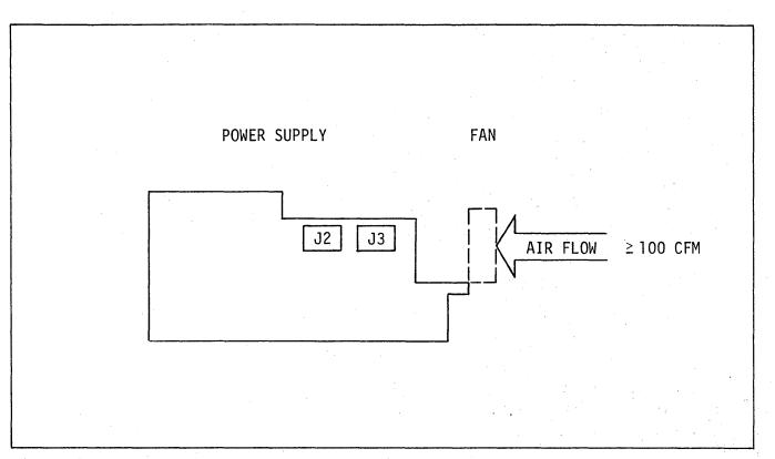
Figure 5-3. External Fan Placement for Adjustment
