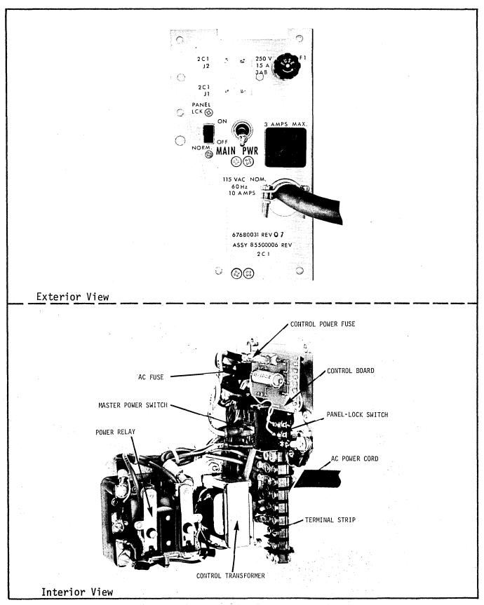
Figure 3-4. 36-A Power Supply AC Power Assembly
