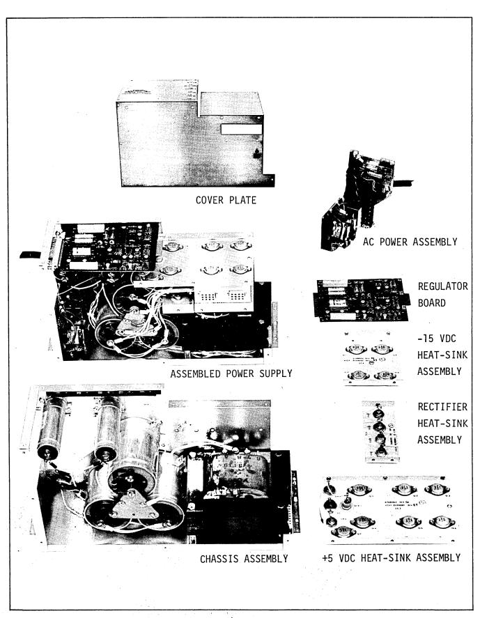
Figure 3-2. 36-A Power Supply Assemblies
