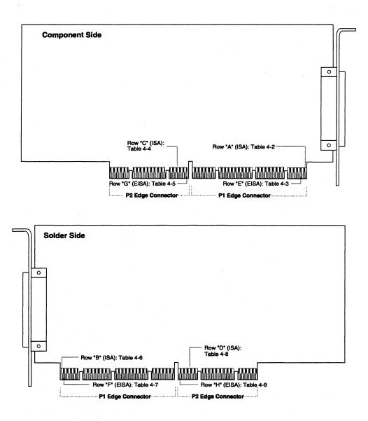
Figure 3-4. Connector Rows on the EISA host adapter's Board Edge
