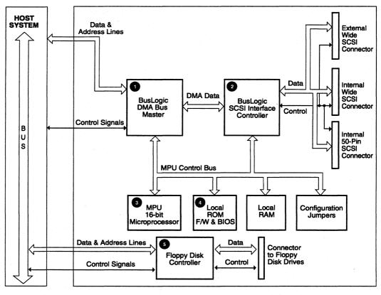
Figure 1-3 is a functional block diagram of the BusLogic adapter. The paragraphs that follow describe the numbered components in the figure.
