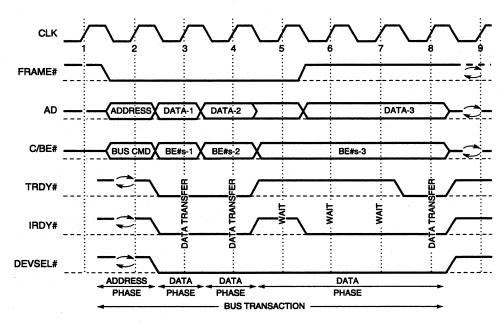
Figure 2-5. Basic Write Operation
