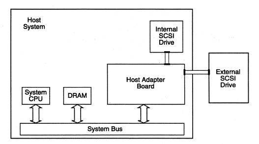
Figure 1-2. System Architecture
