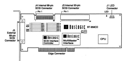
Figure 2-2. The BT-956CD Host Adapter
