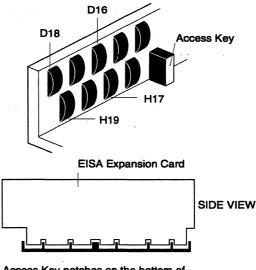
Access Key notches on the bottom of the EISA host adapter card match the Access Keys in the EISA connector.
