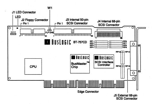
Figure 3-2. The BT-757CD Host Adapter
