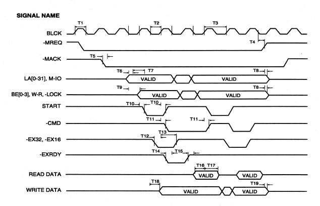
Figure 3-5. EISA Read Cycle Timing Characteristics
