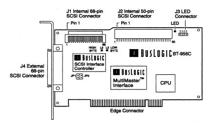
Figure 2-1. The BT-956C Host Adapter
