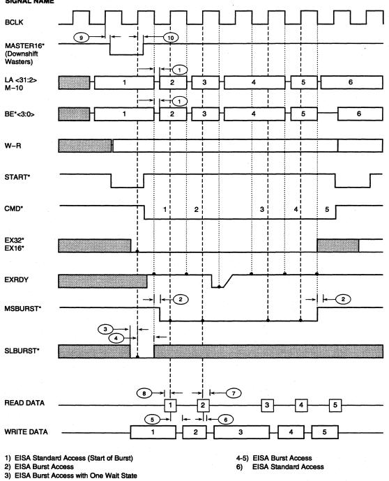
Figure 3-7. EISA 32-bit Burst Cycle Timing Characteristics
