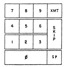
Figure 4-3. 10-Key Auxiliary Keyboard
