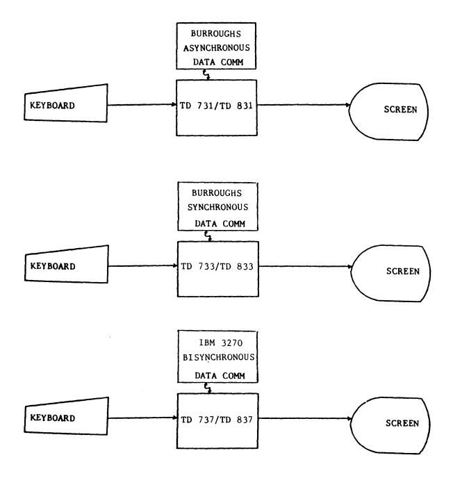
Figure 1-3. TD 730/TD 830 Basic System Configurations
