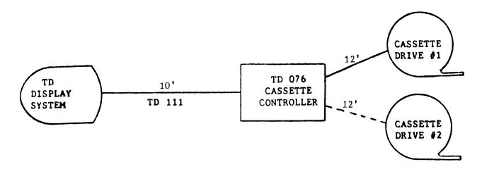
Figure 7-1. Single TD/Cassette Controller Configuration
