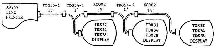
Figure 6-1. TD/A 9249 Configurations
