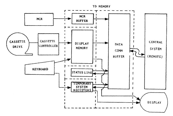
Figure 2=2. Simplified Local Input/ Remote Output Flow
