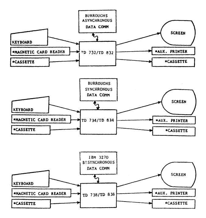
Figure 1-4. TD 730/TD 830 Peripheral Capable System Configurations
