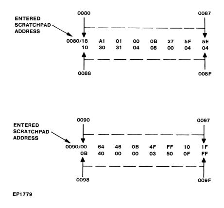
Figure A-1. Display Format of Configuration Area of Scratchpad Memory
