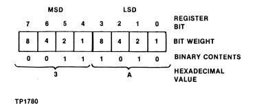
Figure A-2. Interpretation of a Typical Scratchpad Memory Byte
