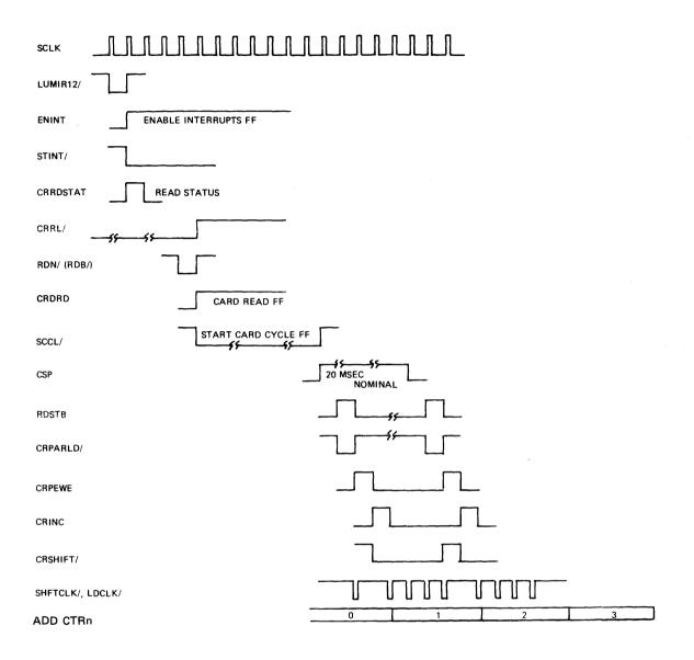
Fig. II-2 BUFFER LOAD TIMING, FIRST COLUMN
