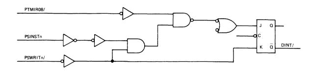
Fig. II-6 DINT FROM LOAD BUFFER CONTROL WORD
