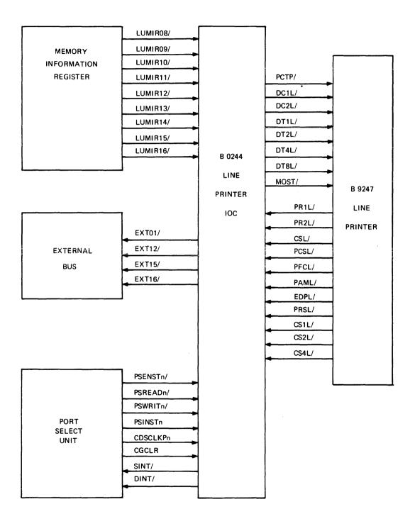
Fig. I-1 INTERFACE BLOCK DIAGRAM
