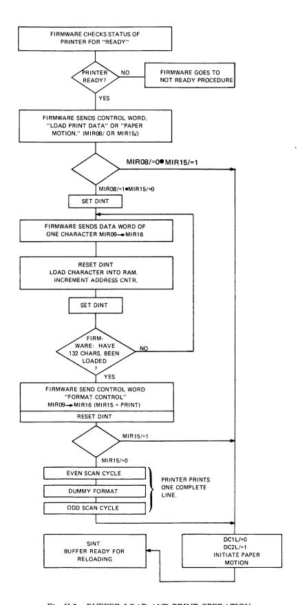
Fig. II-3 BUFFER LOAD AND PRINT OPERATION
