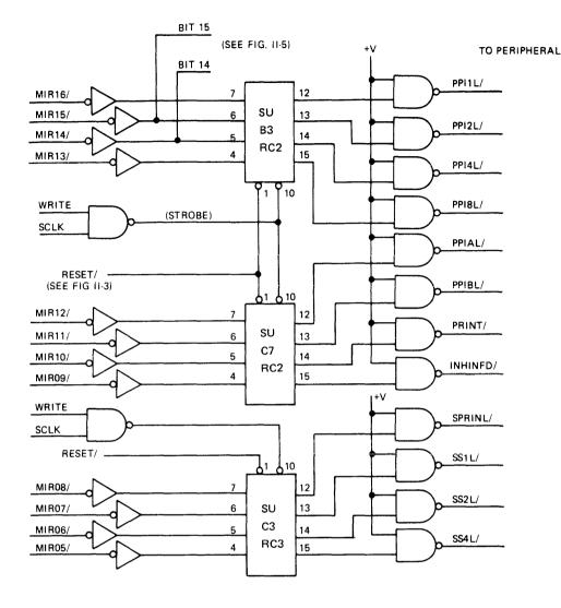
Fig. II-2 MOTION BITS/DATA BUFFER
