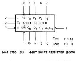
Fig. III-7 SU 4-BIT SHIFT REGISTER
