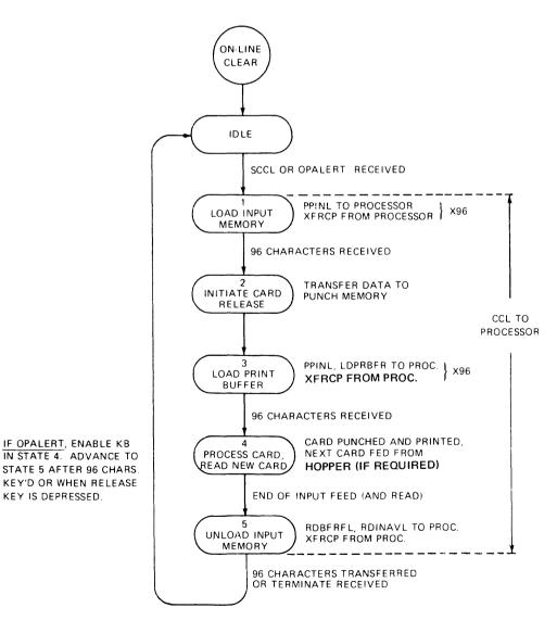
Fig. II-1 A9419 ON-LINE CONTROL COUNTER STATES
