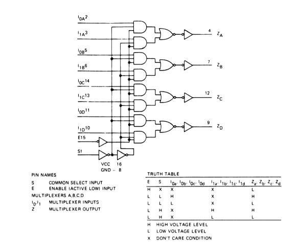
Fig. III-6 S2 QUAD 2-INPUT MULTIPLEXOR, FUNCTIONAL LOGIC AND TRUTH TABLE
