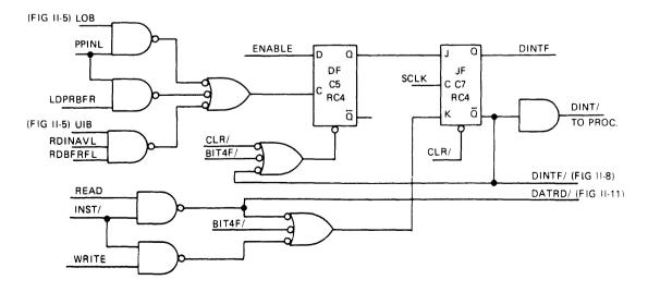
Fig. II-7 DATA INTERRUPT CONTROL
