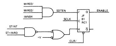
Fig. II-6 INTERRUPT ENABLE FF
