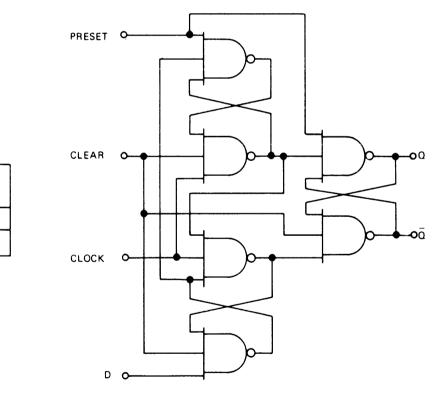
Fig. III-10 DF FUNCTIONAL LOGIC
