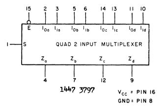
Fig. III-5 QUAD 2-INPUT MULTIPLEXOR
