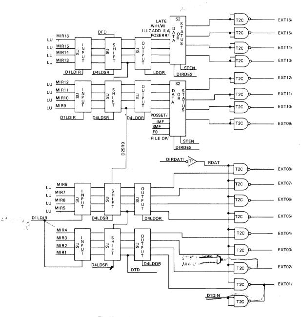
Fig. II-5 INPUT, SHIFT AND OUTPUT REGISTERS
