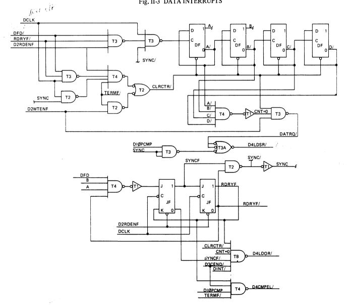
Fig. II-4 SYNC BYTE DETECTOR AND MOD 16 COUNTER
