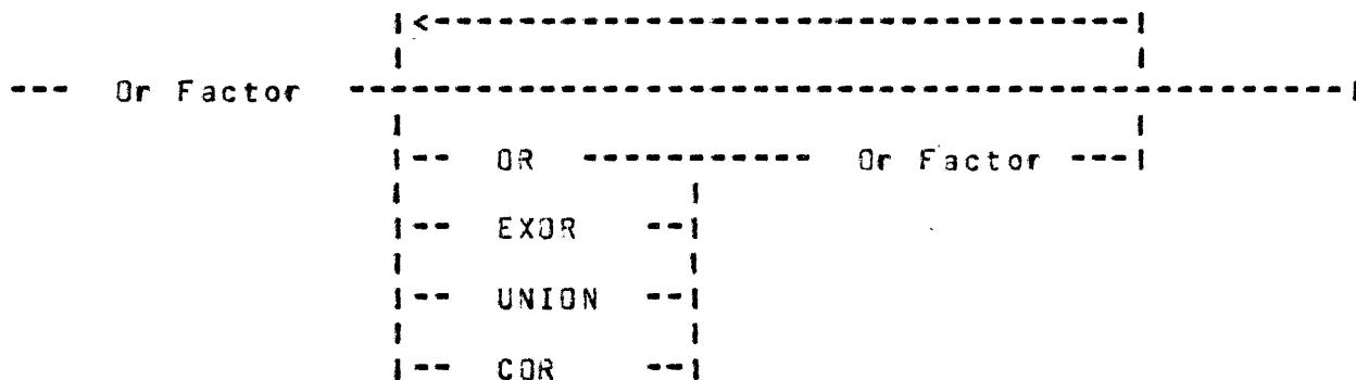
The OR/EXOR operation performs a logical bitwise OR/EXOR of two operands; the result will always be of type Bit. UNION performs a set union of two operands, and is functionally the same as an OR. COR perfomes a short-circuited OR of two operands. If the first operand is True, the result is True and the second operand is not evaluated. If the first operand is False, the result is the value of the second operand.
