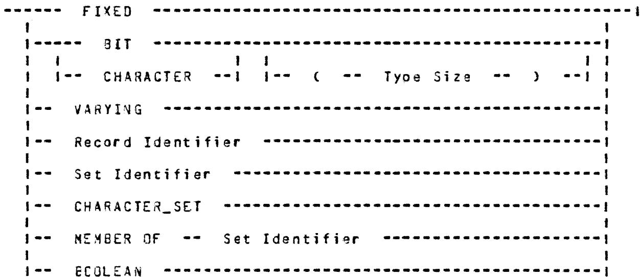
The type FIXED will allocate a 24 bit field, where the high order bit is interpreted as the sign bit (0 = positive, 1 = negative). Negative values are represented in their two's complement form. Fixed numbers can range from  $-(2^{23})+1$  to  $(2^{23})-1$ .
