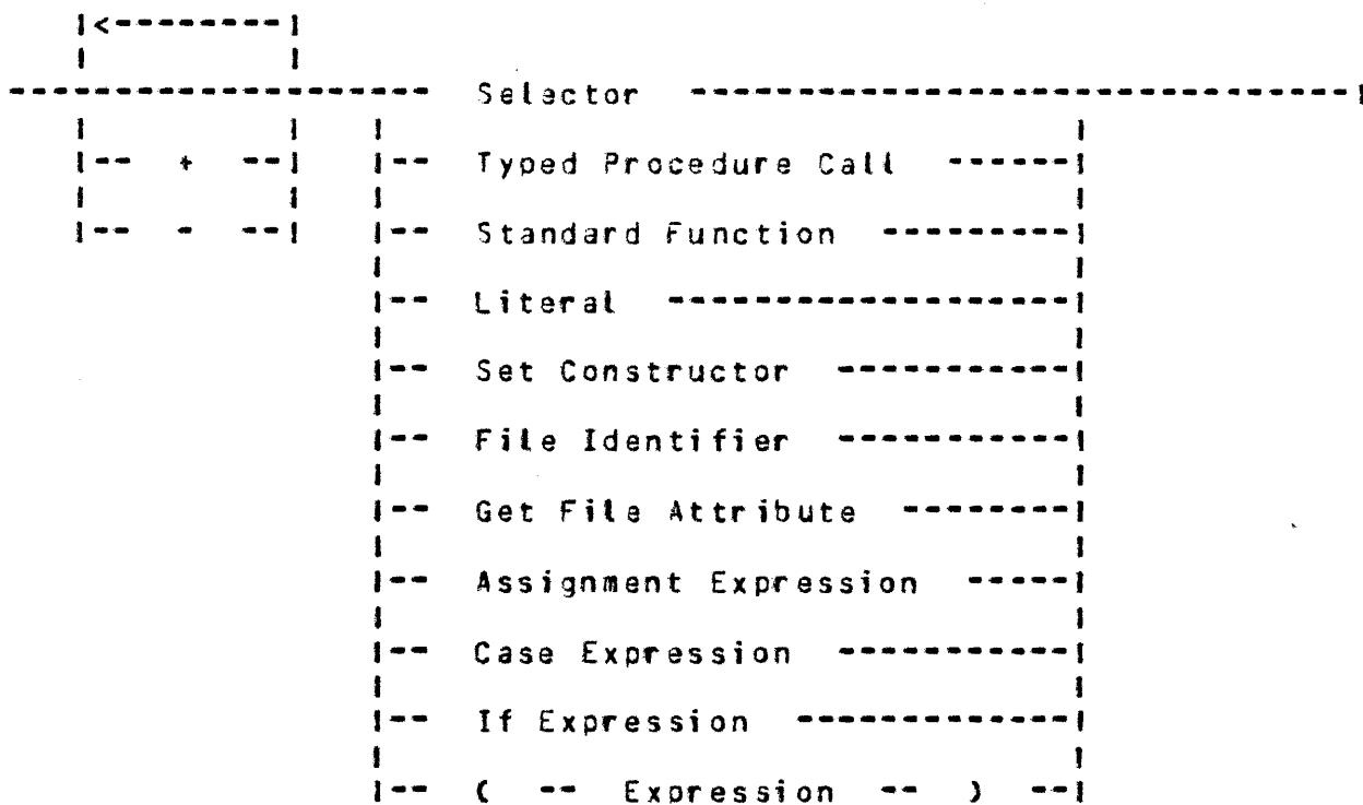
The unary - operation will negate the value of an operand. The unary + does not change the operand.
