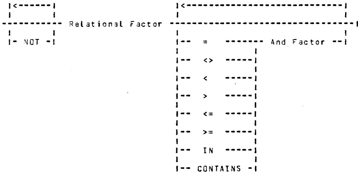
The relational operators leave a result that has a value of 1 if the condition is true or 0 if the condition is false. The NOT operator will perform a logical NOT on one operand, and will have the same type as its single operand.
