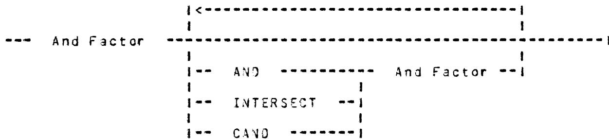
The AND operation performs a logical bitwise AND of two operands; the result will always be of type Bit. The INTERSECT operation performs a set intersection of two operands and is functionally the same as an AND. CAND performs a short-circuited AND of two operands. If the first operand is False the result is False and the second operand is not evaluated. If the first operand is True, the result is the value of the second operand.
