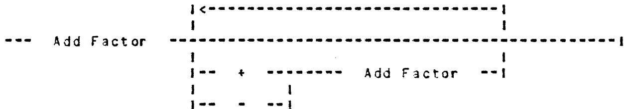
The + and - operations perform 24 bit, two's complement arithmetic on two operands. If either operand is longer than 24 bits, only the rightmost 24 bits will be used. The result will be Fixed if both operands are Fixed, otherwise it will be a Bit(24).
