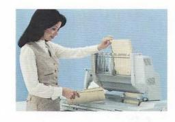
Line Printers. High-output line printers provide even more productive management report writing capabilities. Also, daily tasks — such as invoices and accounts receivable statements — are completed quickly and efficiently. L 9000 programs written for optional line printers can operate on the console matrix printer, taking advantage of the bi-directional print capability. A line printer can be added later without program modification.
