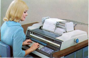
The TC 500 complements its high-speed printing capability with highly automated and flexible forms handling. Forms are spaced 6 lines per inch at speeds up to 20 lines per second. No external tapes or other mechanical control devices are needed. Spacing is completely controlled by internal programing.
