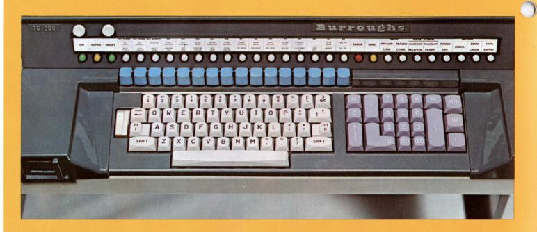
The TC 500 permits complete data input through its *electronic* alphanumeric typewriter and numeric ten-key keyboards.
