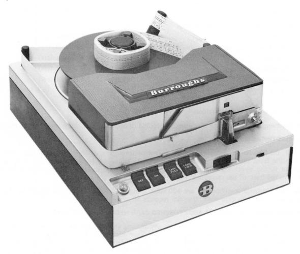
Figure 9.02.00-1 A 562 Punched Paper Tape/Edge Punched Card Perforator
