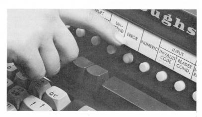
Figure 3.02.00-2 Error Indicator Light, Domestic Data Communication Keyboard, 15½" Forms Handler
