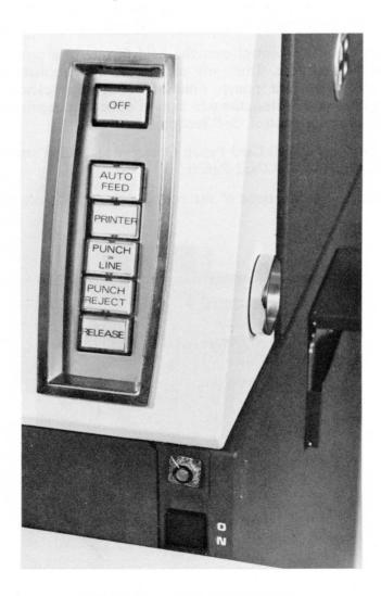
Figure 9.05.01-1 Style A 149 Control Panel
