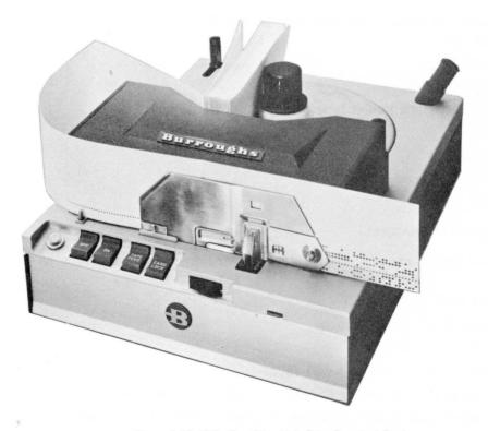
Figure 9.02.13-2 Punching Unit Edge Punched Cards
