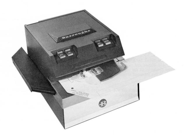
Figure 9.01.15-1 Reading Edge Punched Cards
