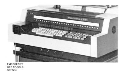
Figure 5.04.00-2 Emergency Switch, Keyboard Printer of TC 700 System
