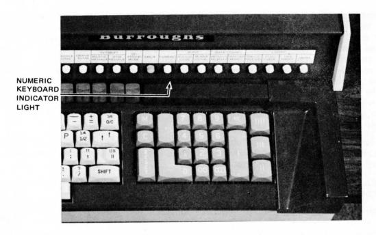
Figure 3.01.00-1 Numeric Keyboard and Indicator Light, 151/2" Forms Handler
