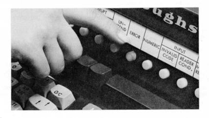
Figure 3.01.00-2 Error Indicator Light, Domestic Data Connumications Keyboard, 15½" Forms Handler
