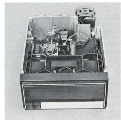
With 1.25 megabytes of fast random access storage, the 9489 is well suited for computer based, transaction-oriented small business systems and intelligent terminals. In the dual drive Master/Slave configuration, the Master connects via an I/O cable to the host and contains additional electronics common to both units. The Master and Slave units are interconnected and allow for seek/overlap operations and a combined storage capacity of 2.5 megabytes.
