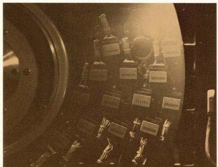
A special, compact disk file Systems Memory acts as a high speed on-line extension of the B 500's main memory. Each data track has its own read/write head. Data switching is completely electronic and is handled at many times the average speed of conventional disk files.
