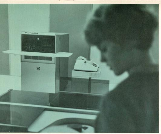
The B 500 is available in punched card, magnetic tape, disk file, and data communications configurations. And it comes with a broad line of cost-conscious peripherals that include a new printer and Burroughs unique "clustered" magnetic tape units.
