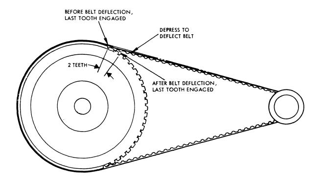
Figure 6-5. Reel Servo Belt Tension Adjustment
