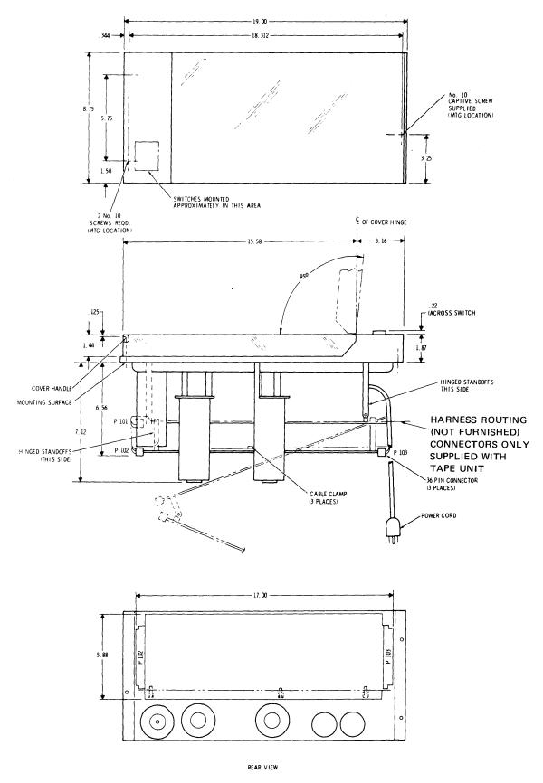
Figure 2-3. Installation Diagram
