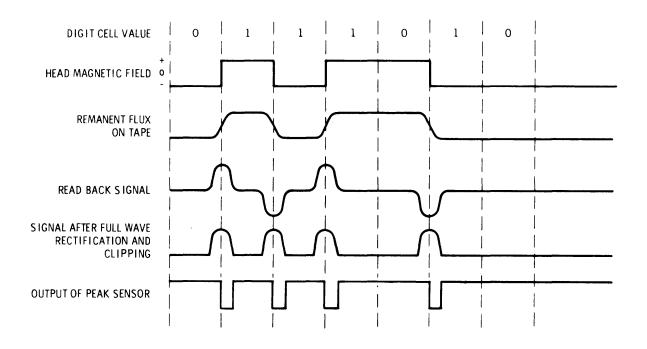
Figure 4-9. Write and Read Waveforms
