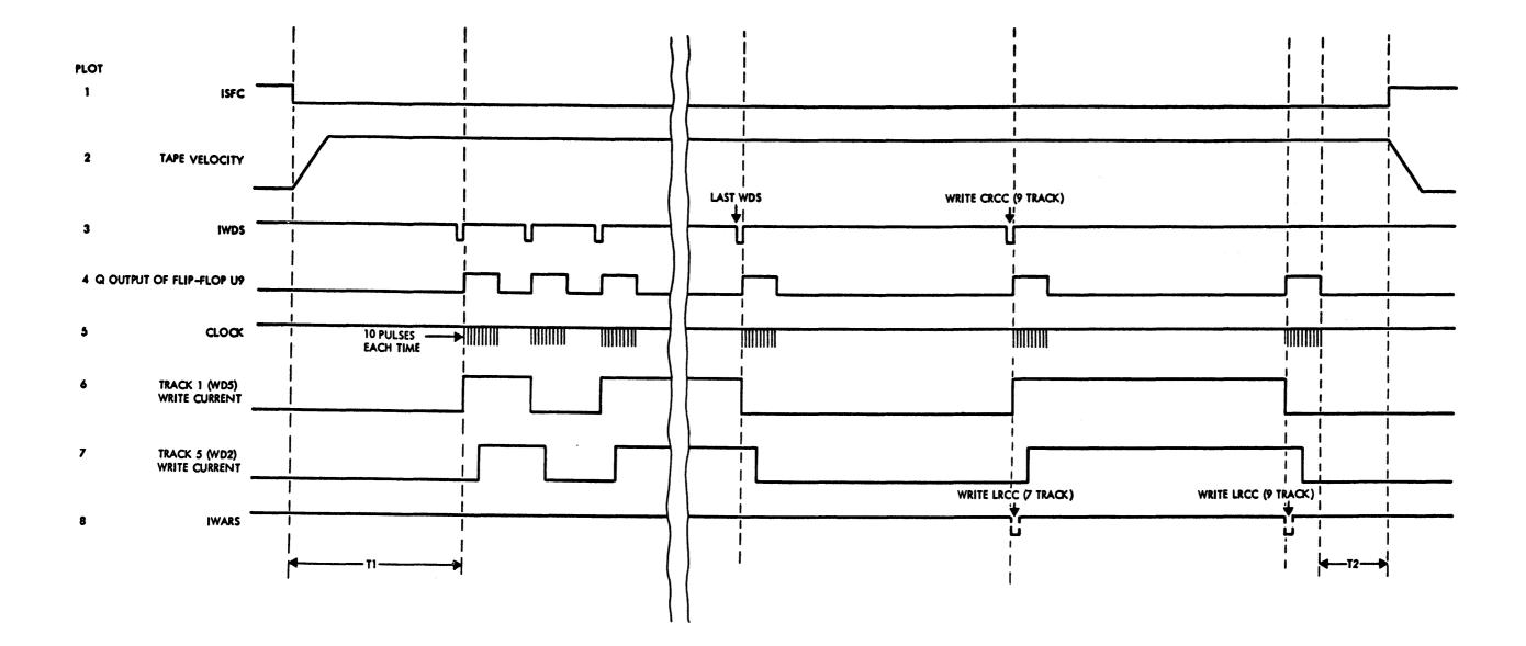
Figure 4-22. Timing Diagram, Data Recording
