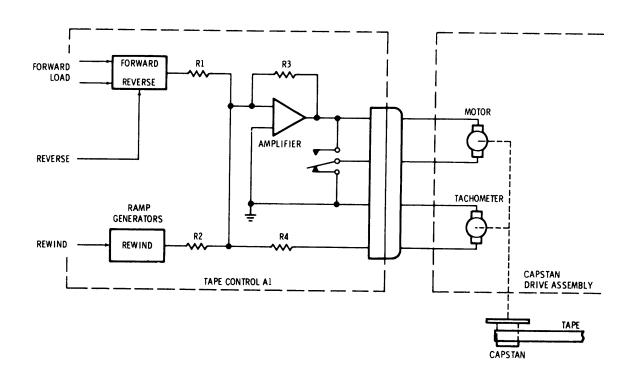
Figure 4-4. Capstan Servo Block Diagram
