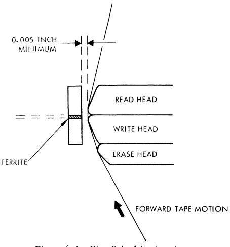
Figure 6-9. Flux Gate Adjustment
