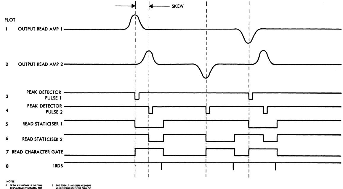
1. SKEW AS SHOWN IS THE TIME DISPLACEMENT BETWEEN THE READ SIGNALS FROM THE TWO TRACKS.
