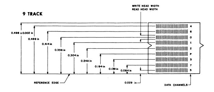
Figure 4-7. 9-Track Allocation and Spacing
