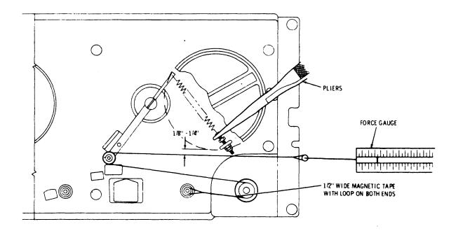
Figure 6-8. Tension Adjustment for Take-up Reel
