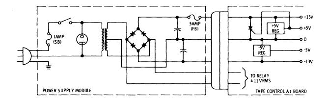
Figure 4-2. Block Diagram of Power Supplies
