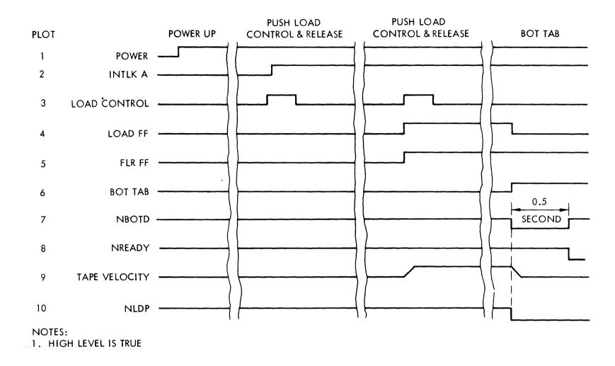
Figure 4-19. Tape Control Waveforms During Load Sequence
