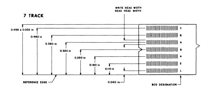
Figure 4-8. 7-Track Allocation and Spacing
