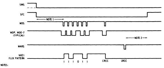
1. Pre-record delay should be calculated to produce 3.5 inches of travel when starting from BOT; otherwise 0.4 inch in a 9-channel Tape Unit and 0.51 inch in a 7-channel Tape Unit.
