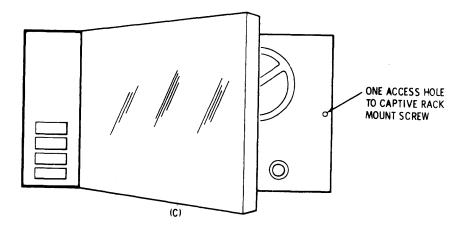
Figure 2-2. Rack Mounting the Tape Unit
