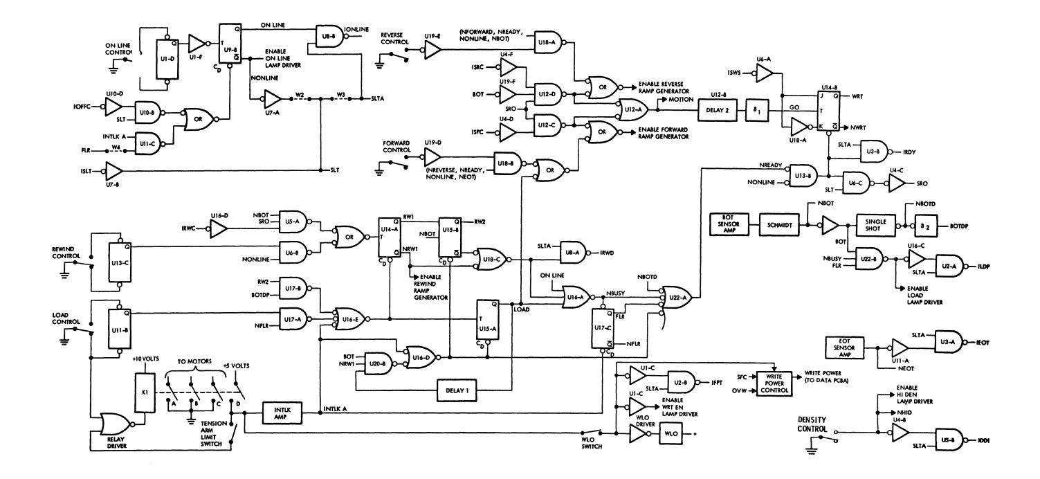
Figure 4-24, Block Diagram, Tape Control Logic
