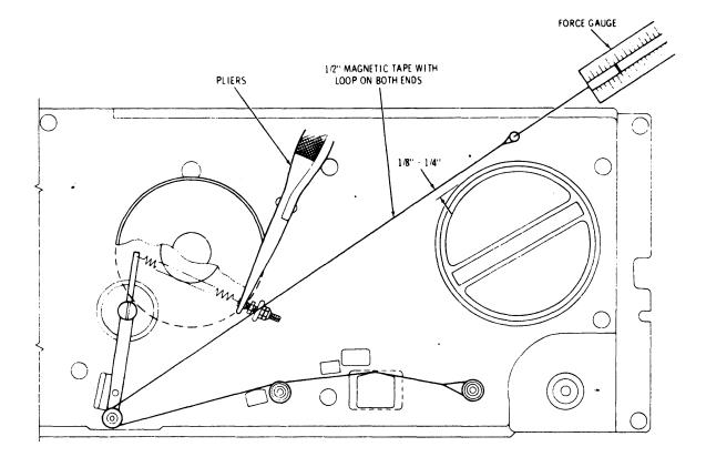
Figure 6-7. Tension Adjustment for Supply Reel
