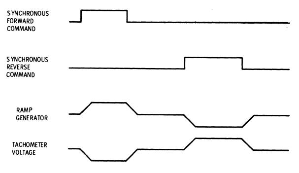
Figure 4-5. Typical Capstan Servo Waveforms
