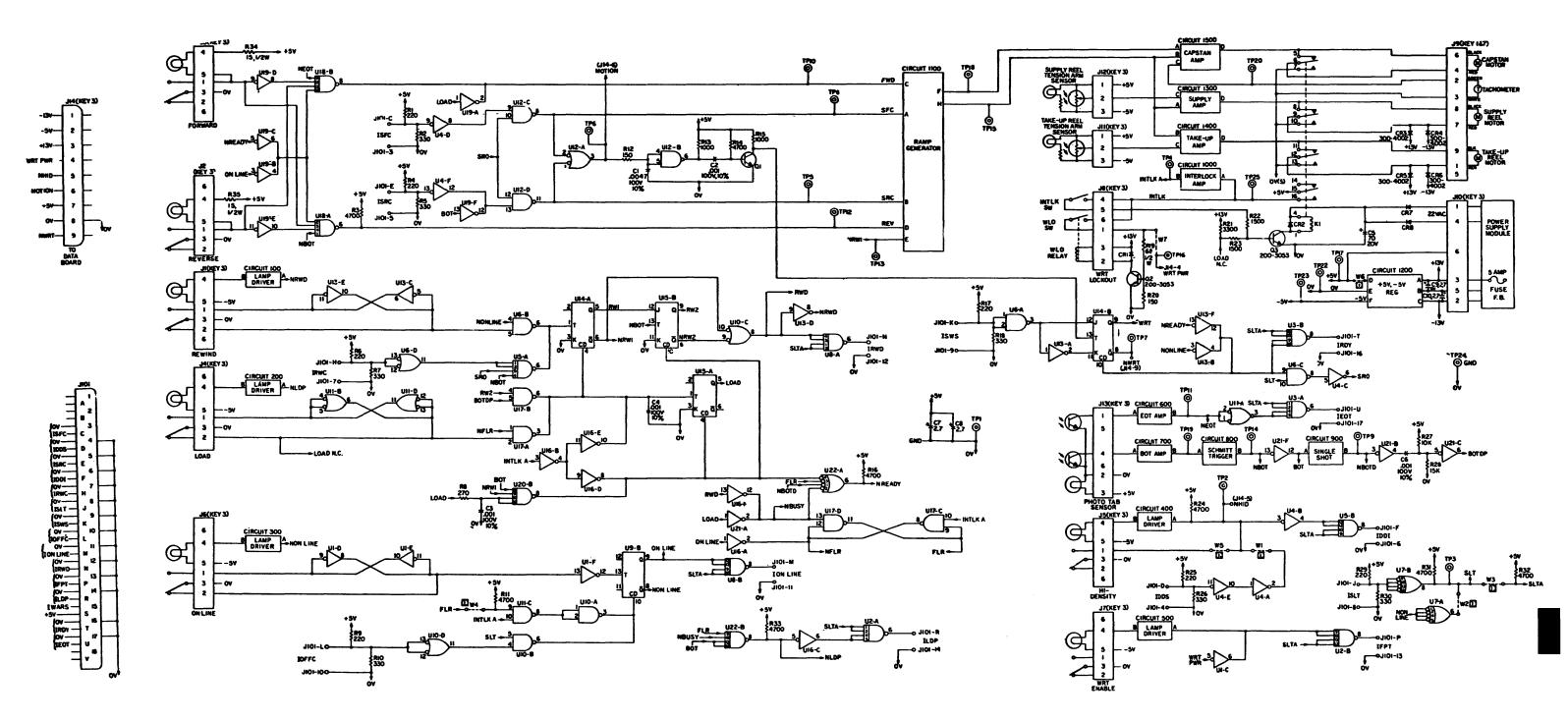
Figure 7-12 Tape Control B2 - Logic Schematics
