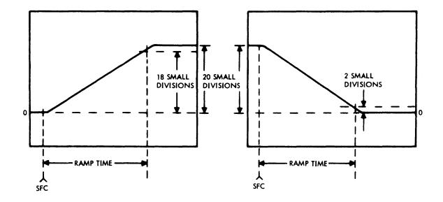
Figure 6-1. Ramp Levels and Timing
