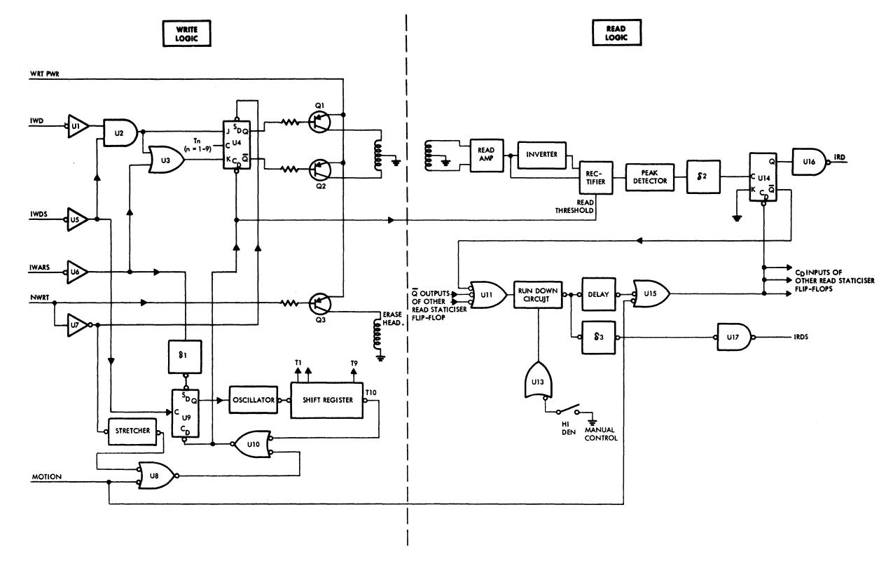
Figure 4-21. Block Diagram, One Channel of Data Electronics
