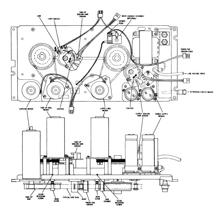
Figure 6-2. Tape Deck Diagram (Rear View)
