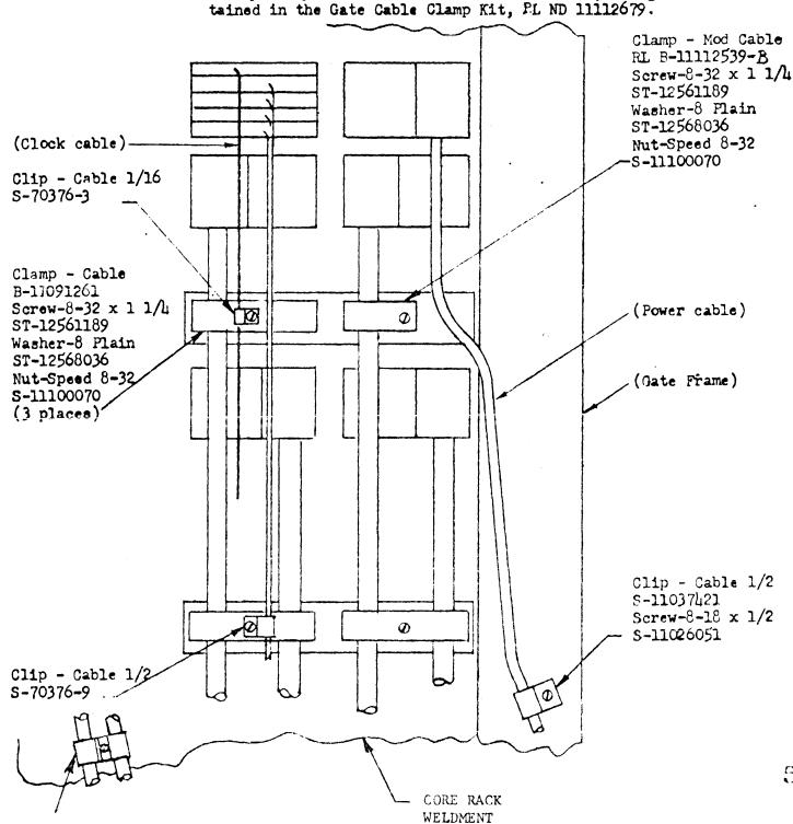
CLIP-CABLE 3/8, S-70376-7 (2 REQ'D) SCREW-8-32 X 1/2, ST-12561122 NUT-8-32 HEX, ST-12565263 WASHER-8 PLAIN ST-12568036 WASHER-8 IT LOCK ST-12567731
