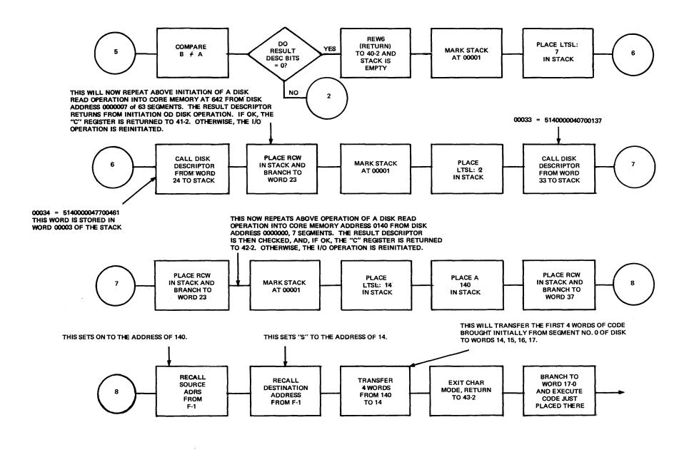
Figure 7-1. Detailed Flowchart of the H/L Card (Sheet 2 of 2)
